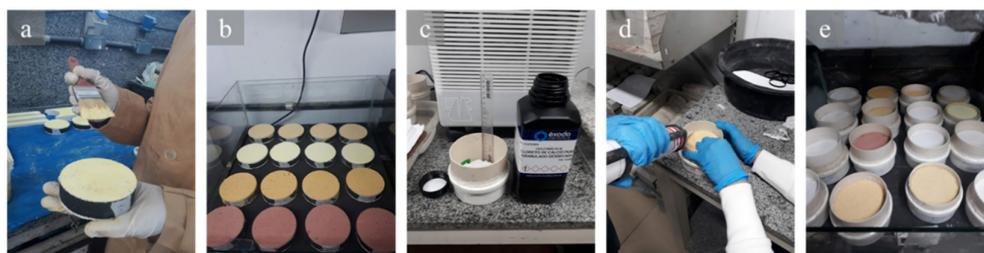
**Figure 1.** (a) Painting the substrates; (b) specimens with sealed sides arranged in the glass chamber; (c) PVC support with calcium chloride desiccant ( $\text{CaCl}_2$ ); (d) sealing the sides of the support with silicone; (e) supports with specimens in the chamber with relative humidity of  $50 \pm 5\%$ .
