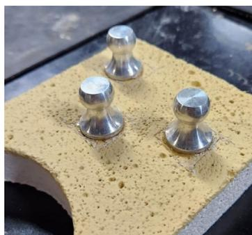
**Figure 2.** Specimen submitted to the adhesion test D4541 [33].
