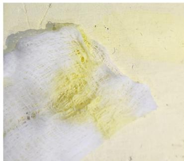
**Figure 4.** Washability of paint specimen with lime + yellow dye formulation.
