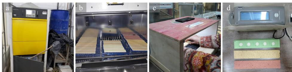
**Figure 3.** (a) Weathering chamber; (b) disposal of specimens inside the weathering chamber; (c) photograph capture; (d) colorimetric analysis using a spectrophotometer.
