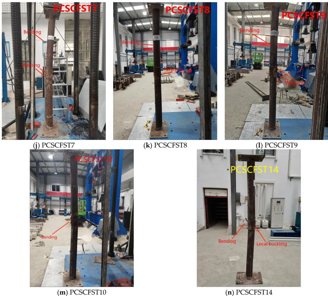
**Figure 6.** Failure phenomena in specimens.
