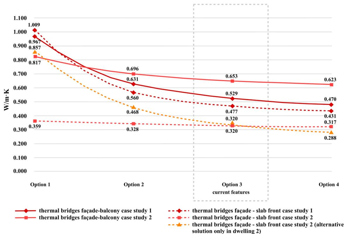
**Figure 18.** The linear thermal transmittance depending on the type of thermal bridge and the thickness of the thermal bridge insulation.
