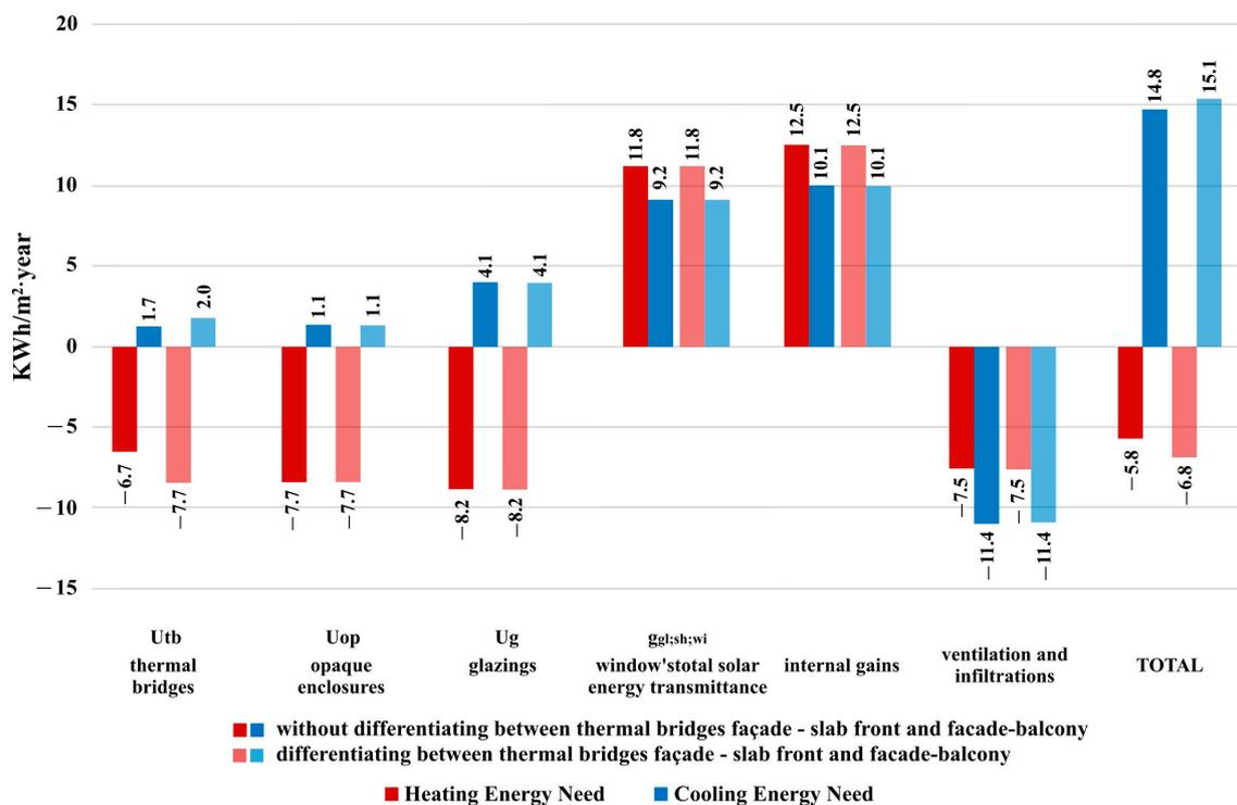
**Figure 15.** Total annual energy needs of dwelling 1 according to the type of thermal bridge.
