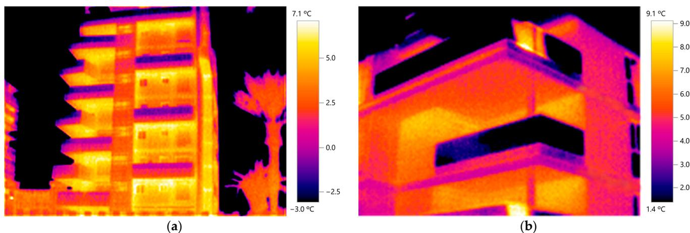
**Figure 11.** A thermographic image of the facades of the two buildings analyzed in detail: (a) case study 1 (brick facade with interior insulation and cladding); (b) case study 2 (facade with ETICS).
