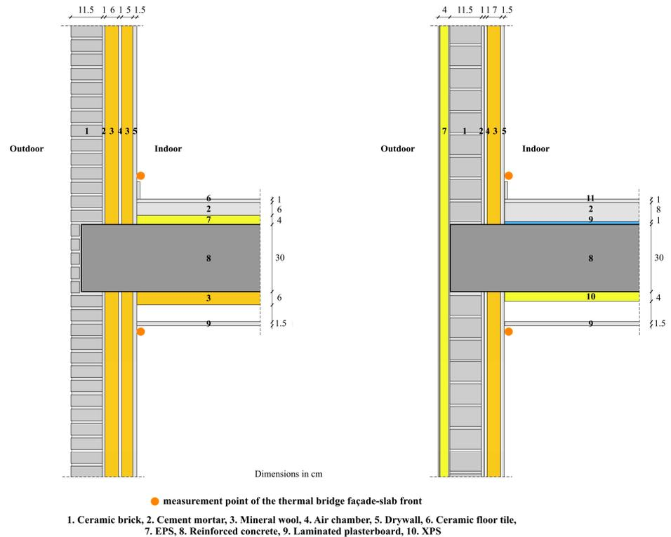
**Figure 6.** Drawings of the facade–slab junction indicating the measurement points: (a) case study 1 (brick facade with interior insulation and cladding); (b) case study 2 (facade with ETICS).
