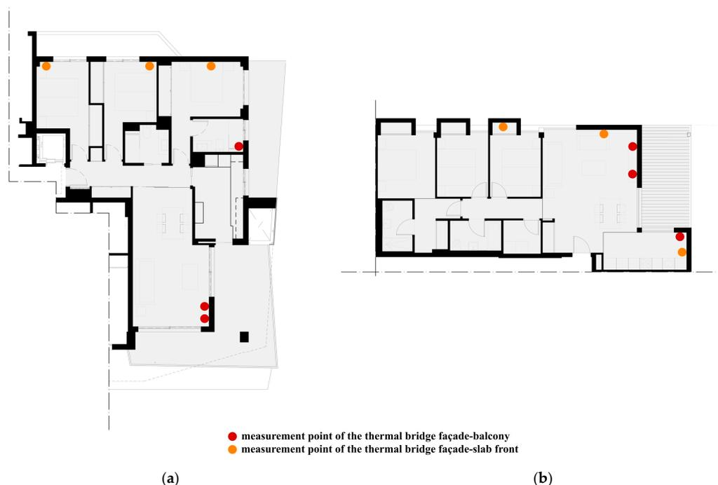
**Figure 5.** Drawings of the two analyzed dwellings indicating the measurement points: (a) case study 1 (brick facade with interior insulation and cladding); (b) case study 2 (facade with ETICS).
