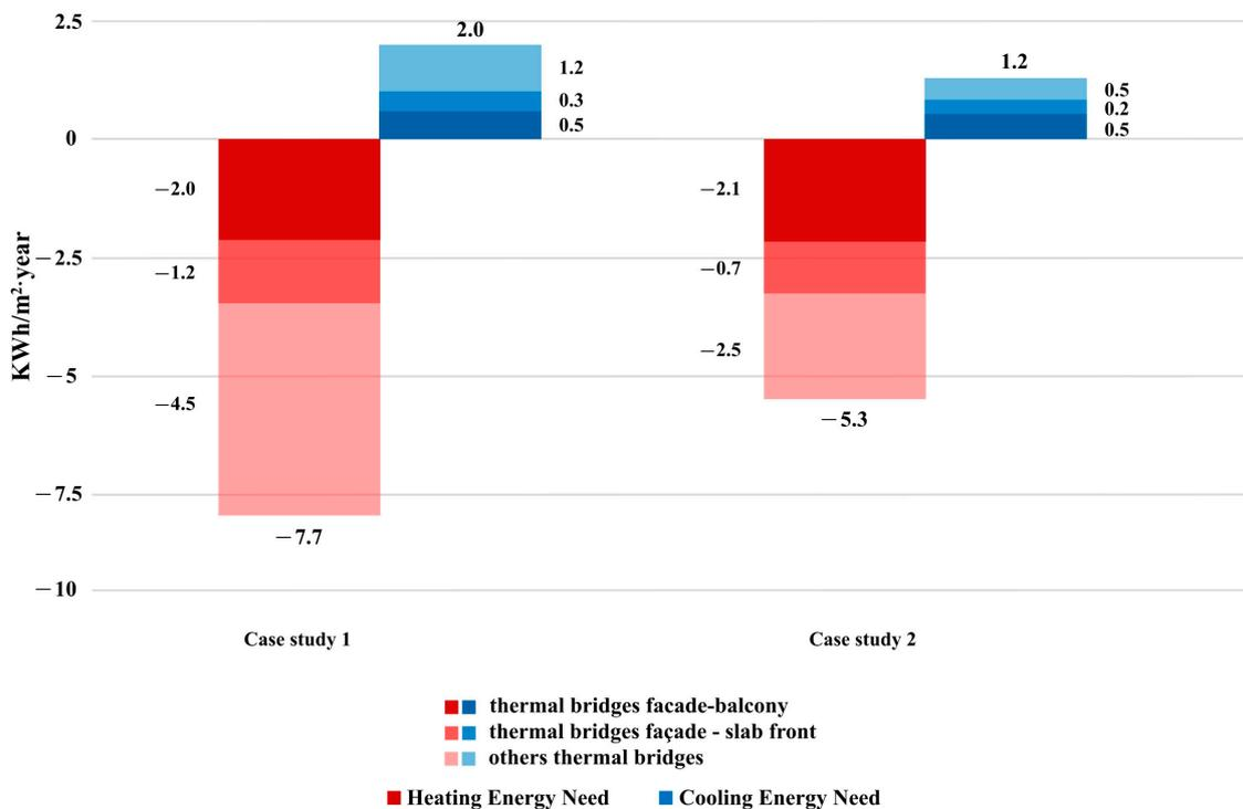
Figure 17. Total annual energy needs according to the type of thermal bridge in each dwelling surveyed.
