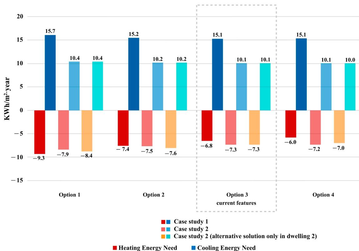
Figure 19. Total annual energy needs according to the thickness of the thermal bridge insulation.
