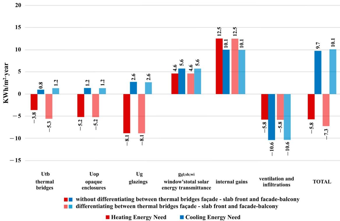
Figure 16. Total annual energy needs of dwelling 2 according to the type of thermal bridge.
