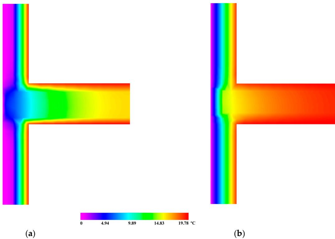
**Figure 13.** Analysis of the linear thermal transmittance by computer simulation according to UNE EN-ISO 10211 of the thermal bridge facade-floor slab front: (a) case study 1; (b) case study 2.
