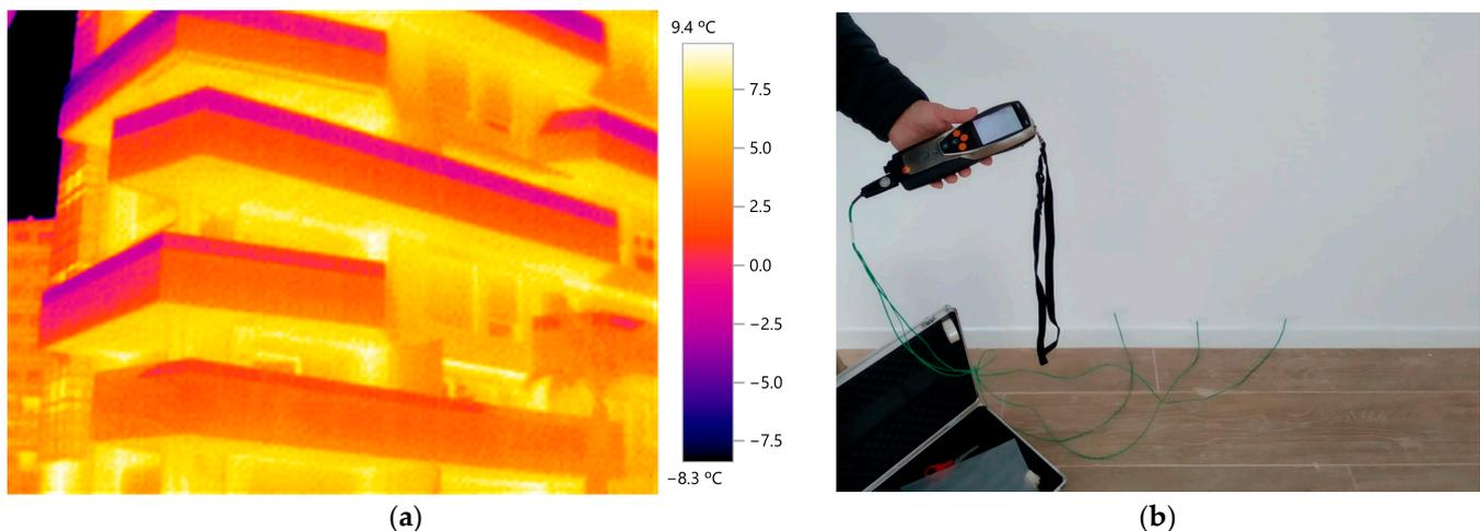
**Figure 1.** On-site measurements of the studied building enclosures: (a) thermographic photograph; (b) thermal transmittance measurement.
