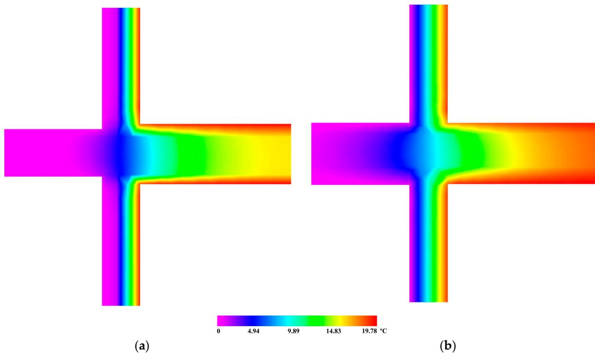
**Figure 14.** Analysis of the linear thermal transmittance by computer simulation according to UNE EN-ISO 10211 of the thermal bridge facade-balcony: (a) case study 1; (b) case study 2.
