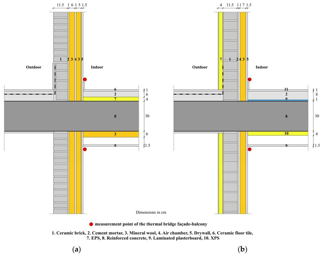
**Figure 7.** Drawings of the facade–balcony junction indicating the measurement points: (a) case study 1 (brick facade with interior insulation and cladding); (b) case study 2 (facade with ETICS).
