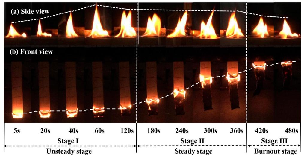
**Figure 2.** (a) Front view and (b) side view image sequences of a typical densified fir flame spread ( $\rho = 896.67 \text{ kg/m}^3$ ).
