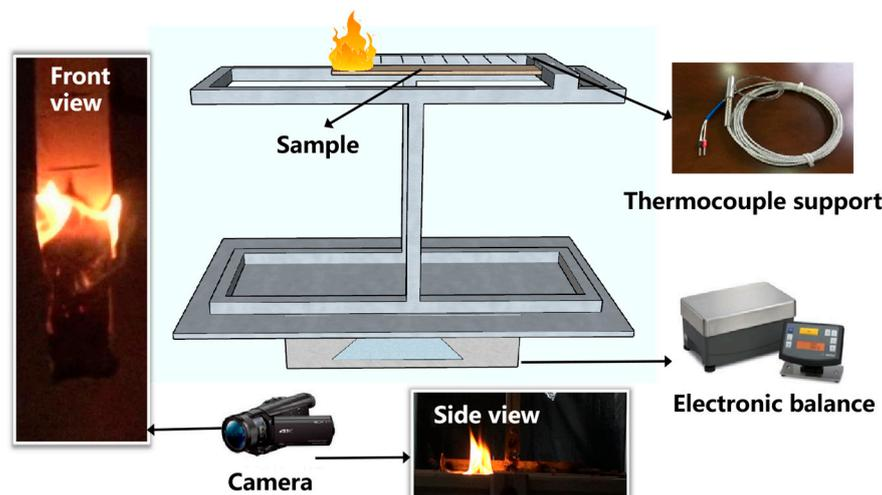
**Figure 1.** Flame spread experimental system schematic.
