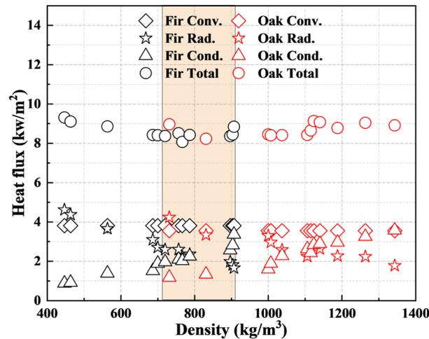
**Figure 10.** Calculated radiative heat, convective heat, conductive heat, and total heat fluxes with different densified fir and densified oak densities. The colored area indicates the overlapped density for both densified wood types.
