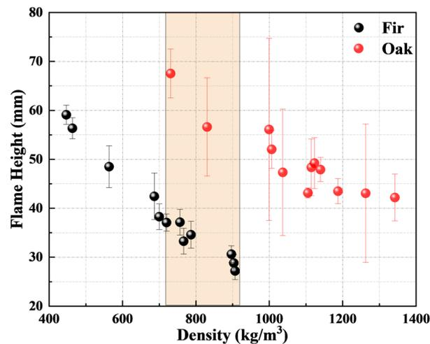
**Figure 6.** Measured flame heights at different densified oak and densified fir densities. The colored area indicates the overlapped density for both densified wood types.
