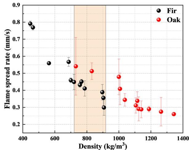
**Figure 3.** Experimental flame spread rates of densified oak and densified fir with different densities. The colored area indicates the overlapped density for both densified wood types.
