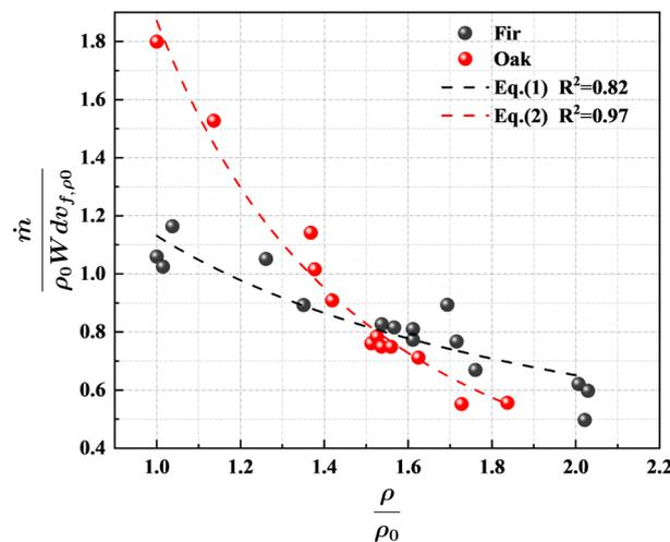
**Figure 5.** Correlation between dimensionless mass loss rates and dimensionless wood densities between densified oak and densified fir.
