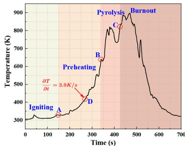
Figure 9. Typical temperature evolution of wood in steady stage (densified oak,  $\rho = 731.20 \text{ kg/m}^3$ ).
