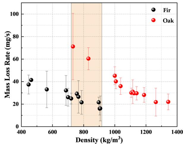
**Figure 4.** The measured mass loss rate of densified fir and densified oak with different densities. The colored area indicates the overlapped density for both densified wood types.
