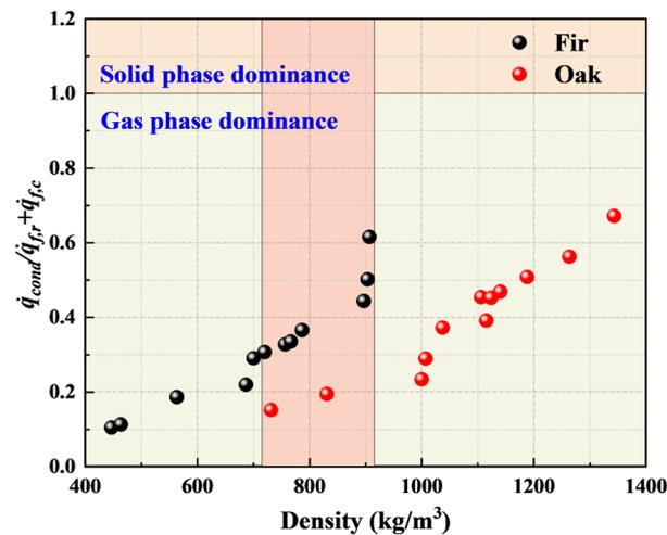
Figure 11. Comparison between the solid-phase and gas-phase heat transfers with different densified fir and oak densities.
