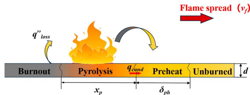
Figure 8. Heat transfer schematic for horizontal flame spread of densified wood.
