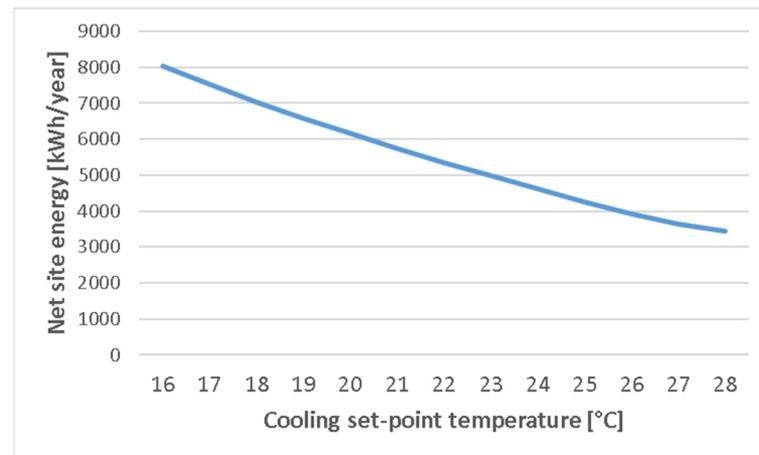
**Figure 8.** Parametric analysis of the net site energy upon variations in the cooling set-point temperature.
