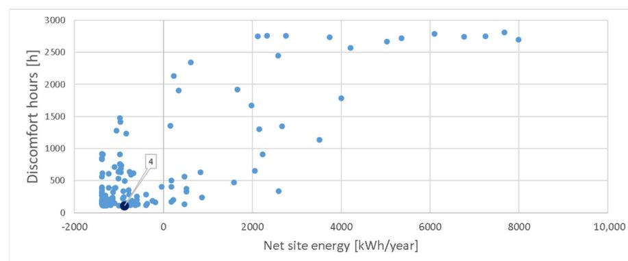
**Figure 14.** Optimal point considering only the combinations using small-sized photovoltaics. The point n°4 indicates the optimal solution.
