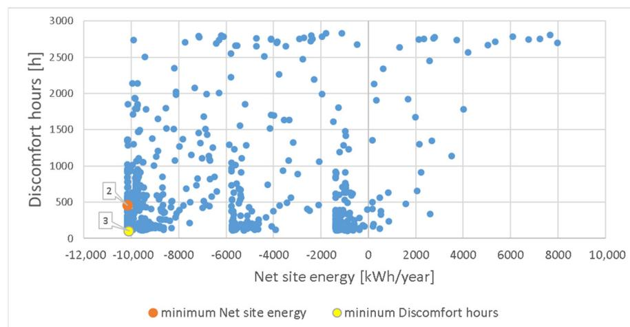
**Figure 12.** Optimization based on the minimization of the net site energy and minimization of discomfort hours ASHRAE 55 Adaptive 80% Acceptability. The points n°2 and n°3 correspond to the solutions with minimum net site energy and minimum discomfort hours, respectively.
