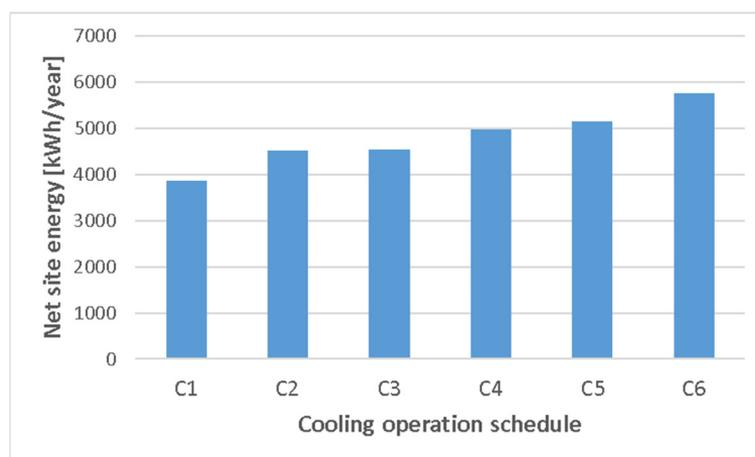
**Figure 7.** Parametric analysis of the net site energy upon variations in the cooling operation schedule.
