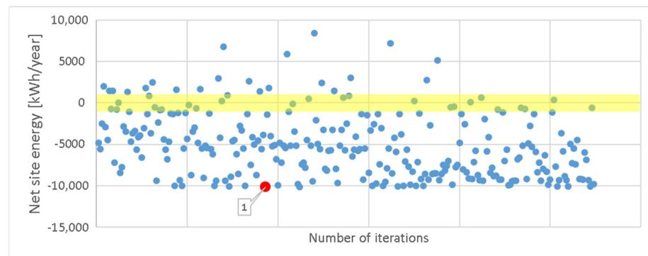
**Figure 11.** Single-objective optimization based on the minimization of the net site energy. The point n°1 indicates the optimal solution. The combinations closest to net “zero” site energy are highlighted with a yellow band.
