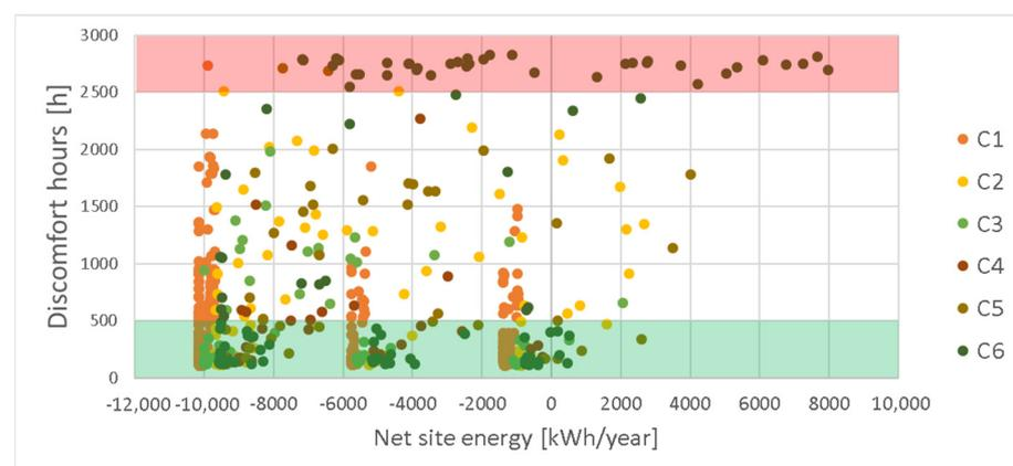
**Figure 15.** Optimization results grouped according to the cooling schedule. The red and green bands represent the solutions with greater and fewer discomfort hours.
