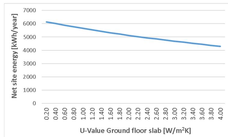
**Figure 5.** Parametric analysis of the net site energy during variations in the thermal transmittance of the ground floor slab.
