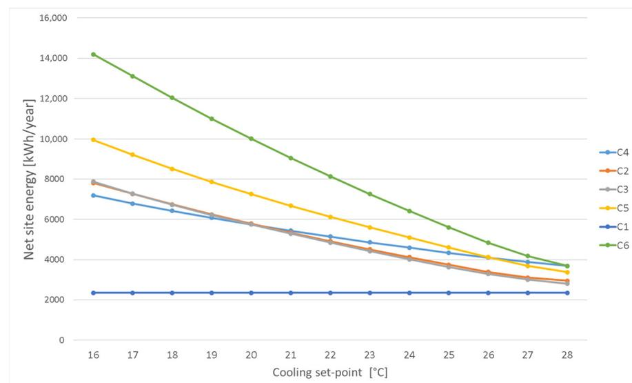
**Figure 9.** Parametric analysis of the net site energy upon variations in the cooling set-point temperature and cooling schedule.
