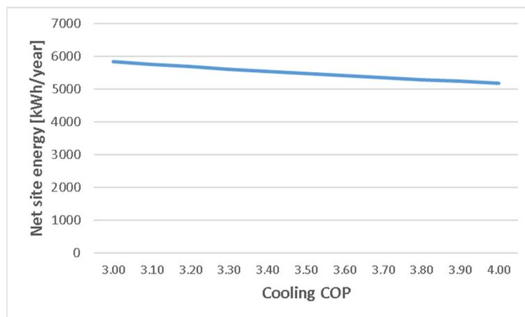
**Figure 6.** Parametric analysis of the net site energy at variations in the cooling COP.
