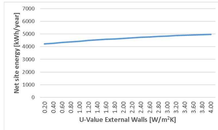
**Figure 4.** Parametric analysis of the net site energy during variations in the thermal transmittance of the external walls.
