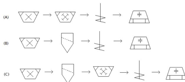
**Figure 1.** Workflow for particle separation: (A) horizontal 2-axis mill followed by hammer mill, particle mixing with binder and pressing; (B) horizontal 2-axis mill followed by sieving for particle separation, mixing, and pressing; (C) horizontal 2-axis mill followed by sieving for particle separation, particle > 1 mm milling with hammer mill, mixing, and pressing.
