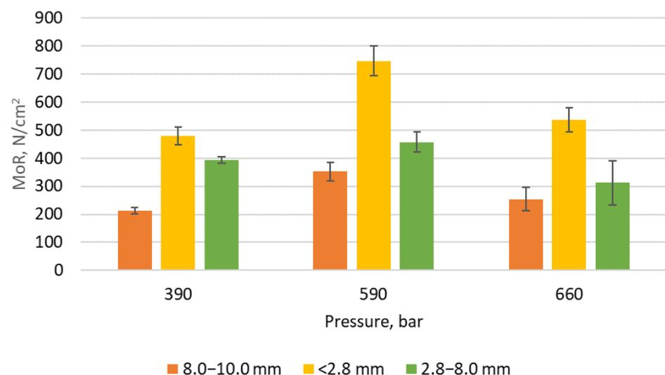
**Figure 2.** Modulus of Rupture depending on pressure and particle size for <2.8 mm particle size boards; 2.8–8.0 mm particle size boards; 10.0 mm particle size boards. Pressing temperature 140 °C. MoR—Modulus of Rupture; error bars represent standard deviation. An analysis of variance (ANOVA) revealed a significant main effect of particle size  $F(2,45) = 41.7$ ,  $p < 0.05$  and pressure  $F(2,45) = 13.1$ ,  $p < 0.05$ , but no significant interactions within  $F(4,45) = 1.80$   $p > 0.05$ .
