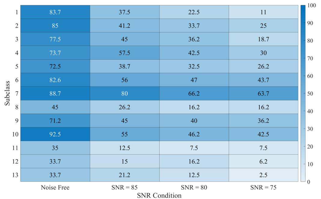
**Figure 12.** The success rate percentage of the LVQ neural network in the defect detection of the gantry crane system in each subclass.
