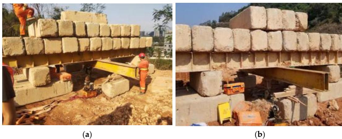
**Figure 4.** Pile bearing capacity detection: (a) No. 8 pile; (b) No. 17 pile.
