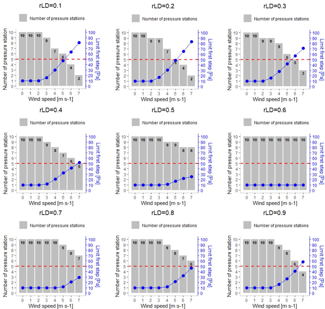
**Figure 10.** Number of pressure tests (stations) for a fan pressurization measurement depending on the wind speed for nine leakage distributions (red line = ISO 9972 constraint with at least 5 pressure stations).
