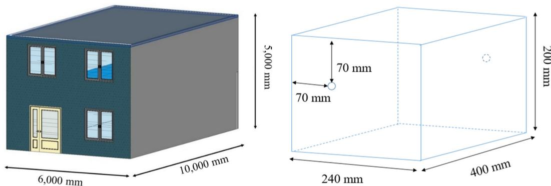
**Figure 3.** Generic two-story house at a real scale (left) and a reduced model at a 1/25 scale (right).
