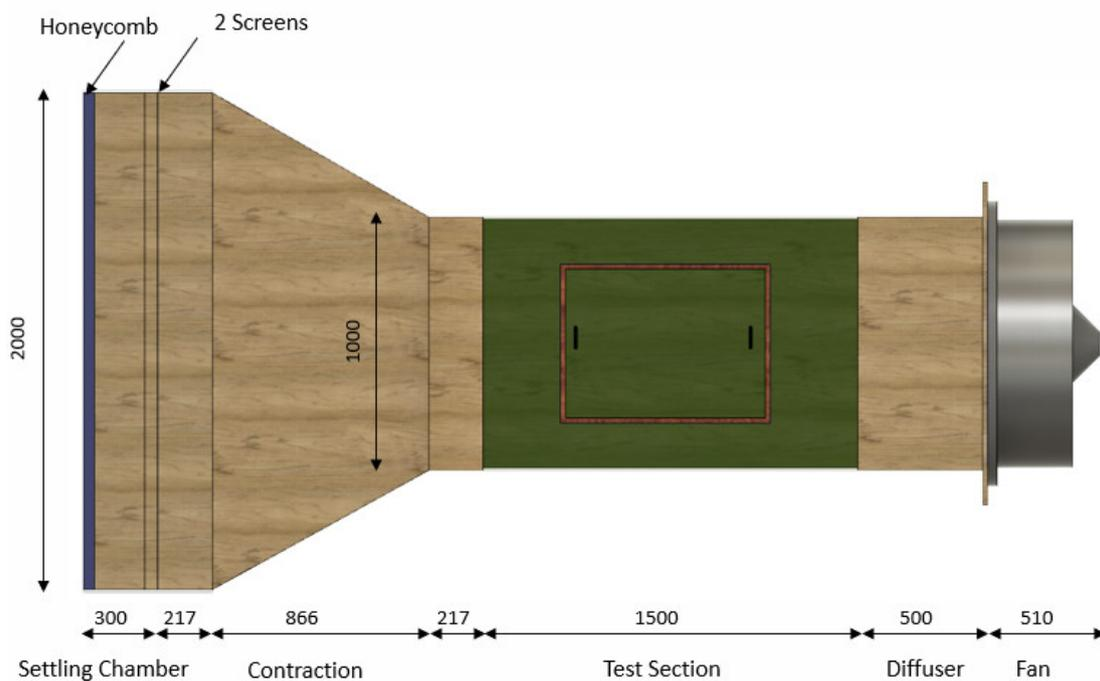
Figure 1. Side view of the final design of the wind tunnel. The dimensions are given in mm.
