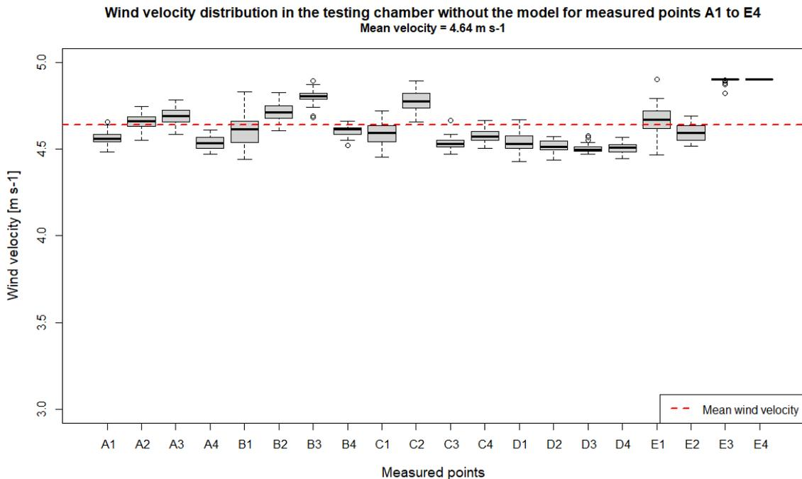
**Figure 9.** Distribution of the wind velocities in the testing chamber for a mean wind velocity = 4.64 m·s<sup>-1</sup>—points A1 to E4.
