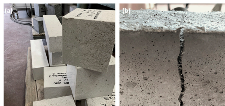
Figure 3. Typical UHPC samples, (a) made of cubes and (b) reinforced with fibres.
