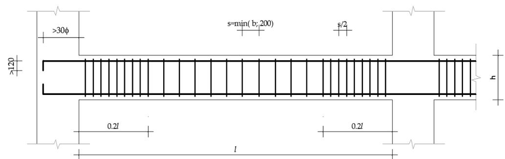
**Figure 7.** Seismic detailing requirements for beams in RC frames according to the PTN-S code.
