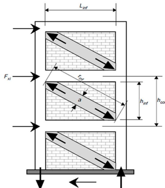
**Figure 26.** A typical RC frame with equivalent diagonal struts.
