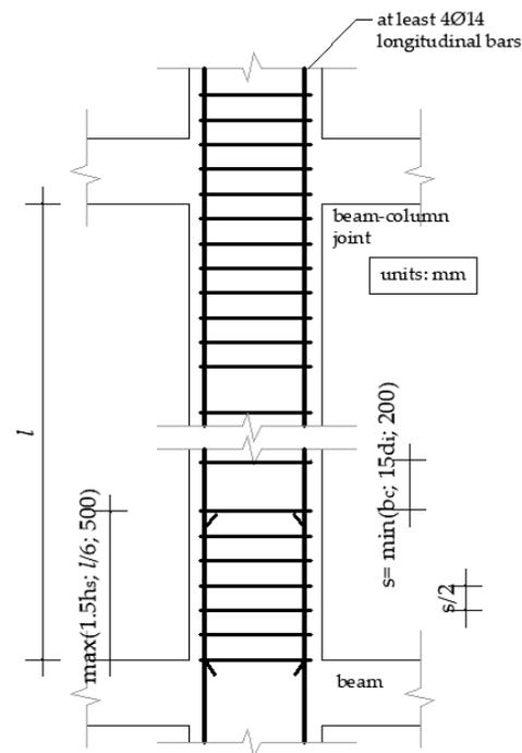
**Figure 8.** Seismic detailing requirements for columns in RC frames in accordance with the PTN-S code.
