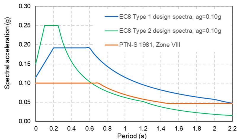
**Figure 12.** Design spectra: Type 1 and Type 2 for Niš, Serbia, according to the EC8-1 ( $a_g = 0.1$  g, ground Type C) and PTN-S codes (zone VIII).
