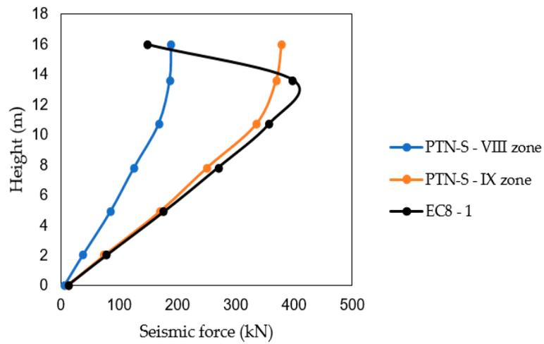
Figure 16. Magnitudes and distributions of seismic forces (Model C).
