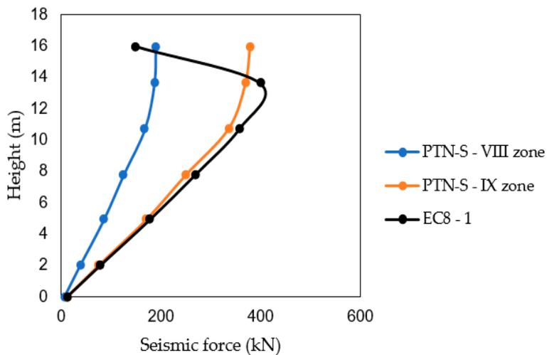
Figure 17. Magnitudes and distributions of seismic forces (Model D).
