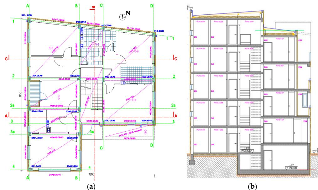
**Figure 11.** Case study building—RC-frame solution: (a) plan at the ground-floor level and (b) vertical section A–A. (This is RC frame structure. Letters and signs in blue color: RC columns of RC frame structure; magenta color: RC beams of RC frame structure and floors).
