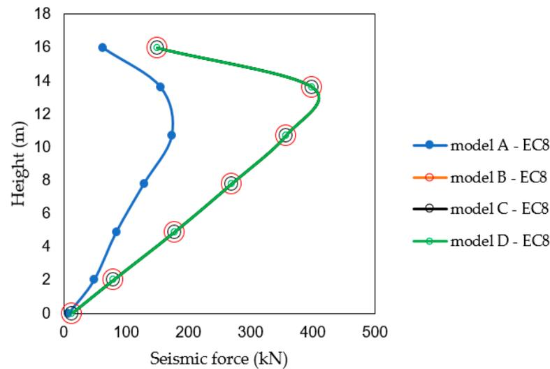
**Figure 19.** Magnitude and distribution of seismic forces for different structure types (A, B, C, and D) determined in accordance with EC 8-1.
