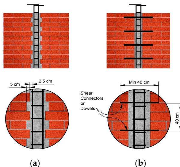
**Figure 5.** Wall-to-tie-column interface: (a) tothing; (b) horizontal steel dowels.
