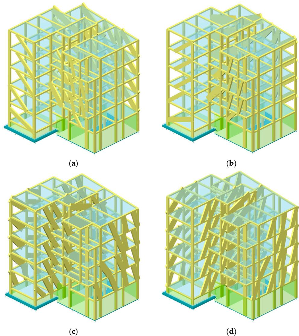
**Figure 27.** Numerical models for RC frames with masonry infills: (a) X1 = X-direction (for seismic forces acting in + direction); (b) X2 = X-direction (for seismic forces acting in opposite direction); (c) Y1 = Y-direction (for seismic forces acting in + direction), and (d) Y2 = Y-direction (for seismic forces acting in opposite direction).
