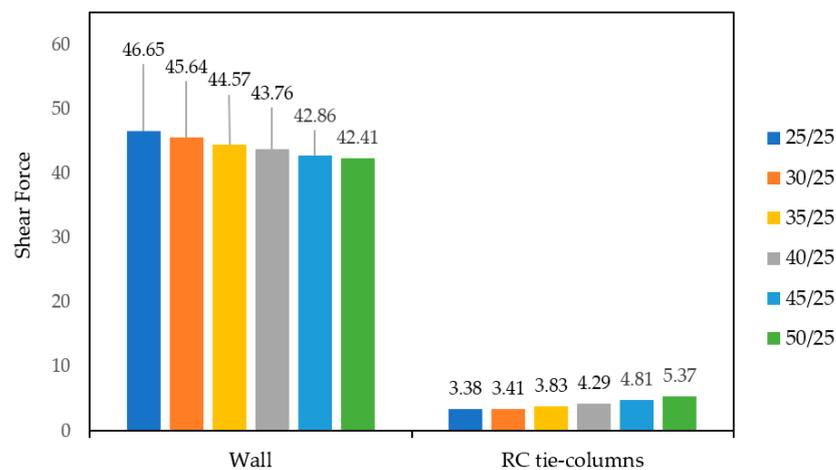
**Figure 24.** Redistribution of the shear force in the structural elements of the CM (masonry and tie-columns) depending on the size of the tie columns.
