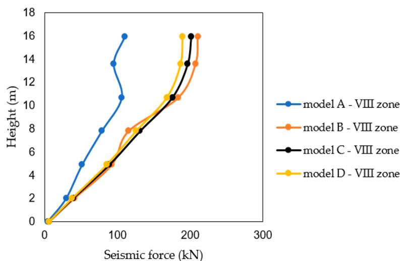
**Figure 18.** Magnitude and distribution of seismic forces for different structure types (A, B, C, and D), determined in accordance with the PTN-S code.
