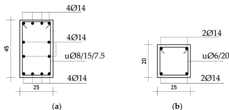
**Figure 28.** Reinforcement details: (a) RC column (RC-frame solution); (b) vertical RC confining element (CM solution).
