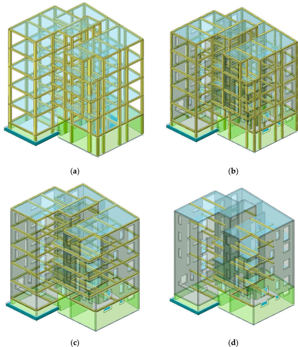
**Figure 13.** Numerical models for different structural systems: (a) Type A; (b) Type B; (c) Type C; and (d) Type D.
