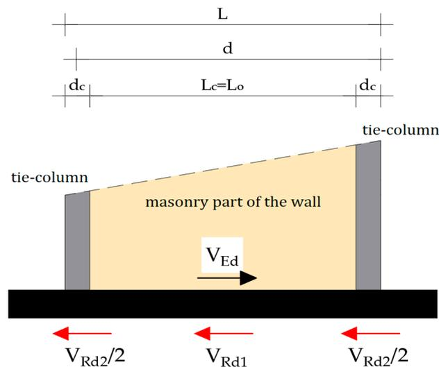
**Figure 21.** Design shear resistance model of a CM wall according to EC8-1.
