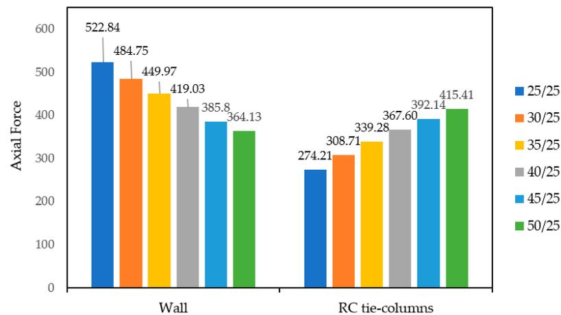
**Figure 25.** Redistribution of the axial force in the structural elements of the CM (masonry and tie-columns) depending on the of the tie-columns.
