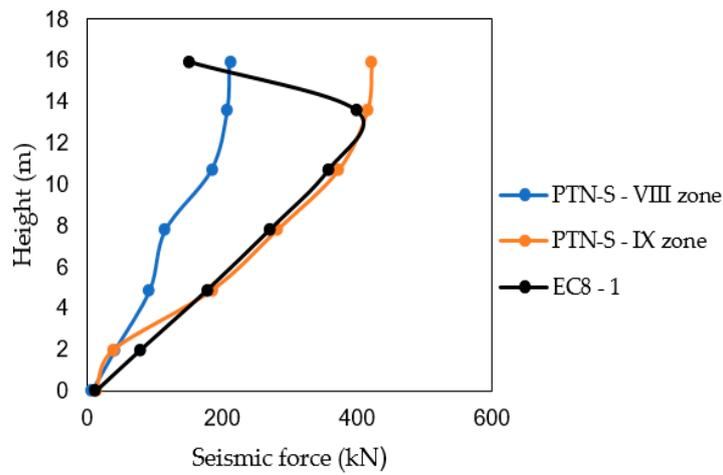
Figure 15. Magnitudes and distributions of seismic forces (Model B).
