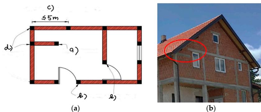
**Figure 4.** Confining elements in CM buildings: (a) a typical floor plan showing the locations of RC tie columns and (b) a discontinuous RC tie beam (an example of an inadequate construction practice). (Red ellipse shows the discontinuity of horizontal confining elements what is serious structural mistake in this case of CM building).
