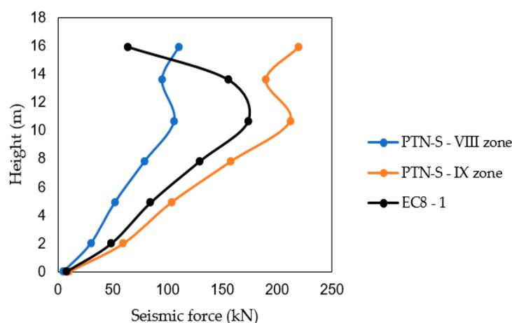
**Figure 14.** Magnitudes and distributions of seismic forces (Model A).
