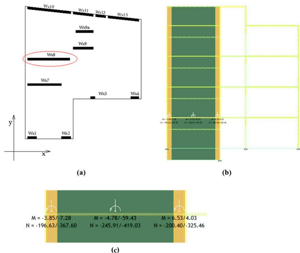
**Figure 22.** Redistribution of gravity and seismic forces in relation to the ground-level wall (WX8) of the case study CM building (Type B): (a) position of the CM wall WX8 (by red ellipse is marked analyzed wall); (b) numerical model of the CM structure with tie-columns of the cross-sectional dimensions 25 cm  $\times$  40 cm; and (c) values of internal forces for the alternative seismic action.
