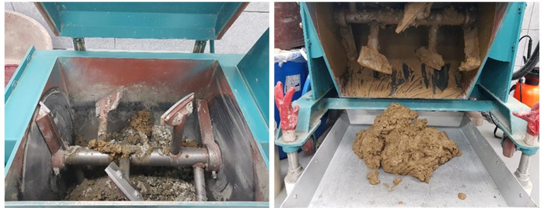
Figure 3. Mixing of CLSM.
