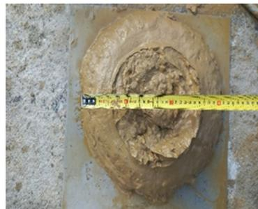
(a) Flow test for backfill CLSM
