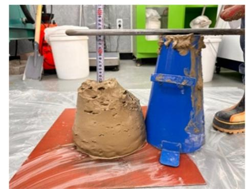
**Figure 9.** Slump test of URHC-6.
