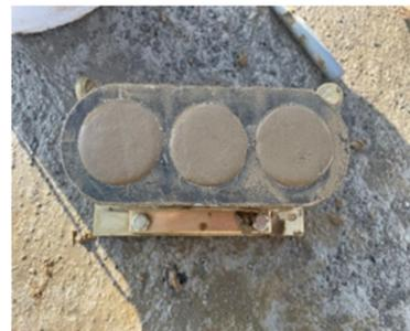
(b) Specimen fabrication for backfill CLSM
