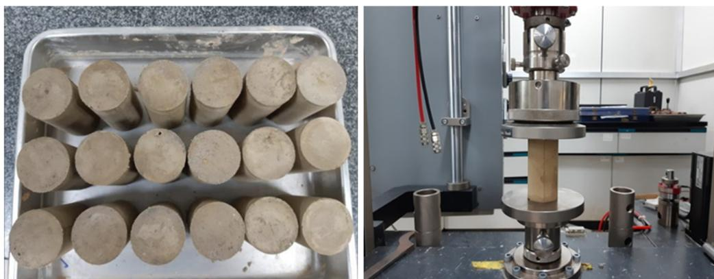
Figure 2. Specimens and test setup for compressive strength test.
