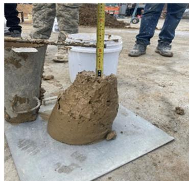
(c) Slump test for subbase CLSM
