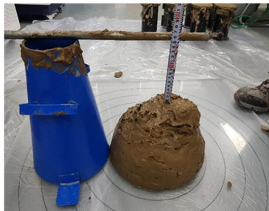
Figure 4. Slump test.
