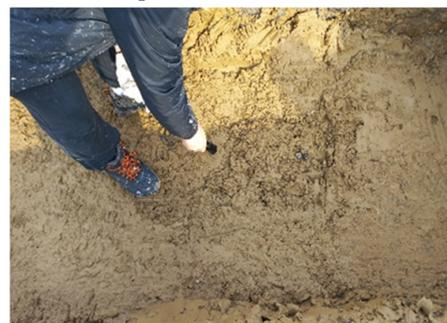
(e) Soil penetrometer test
