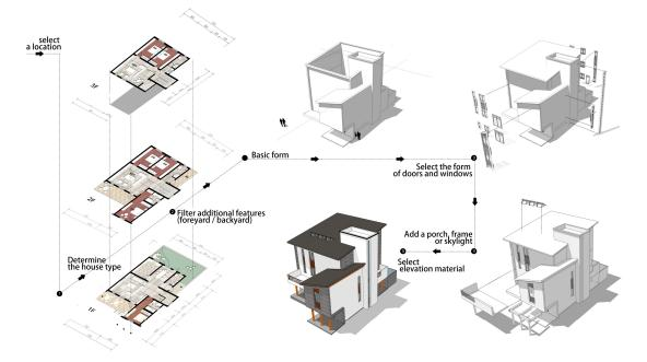
Figure 12. Modularization of the construction process (Layout D).
