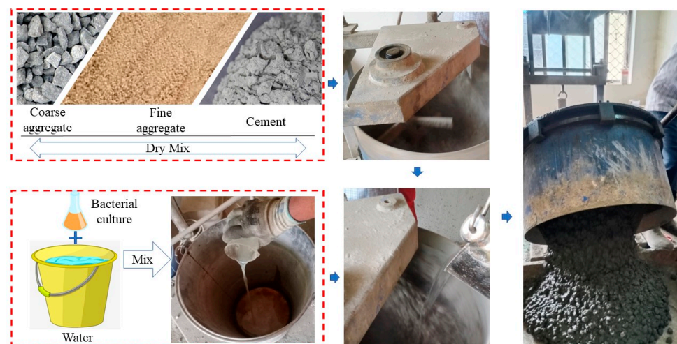
Figure 4. Schematic representation of the concrete mixing procedure.
