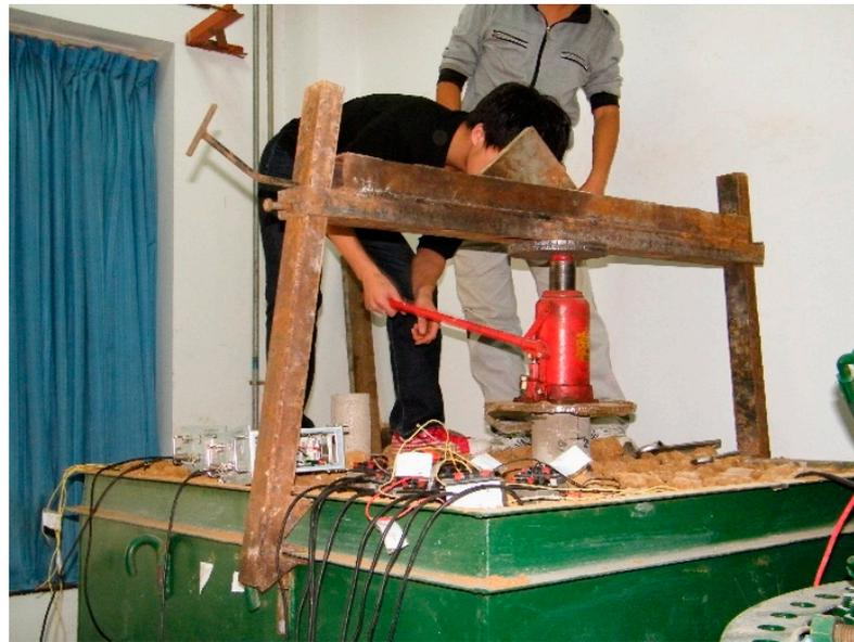
**Figure 3.** Device for reaction beam loading.
