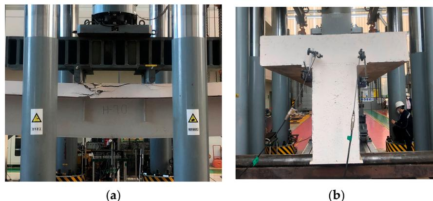
**Figure 4.** Failure modes of the specimens. (a) Concrete crushing of the loading point. (b) Side view of specimen.
