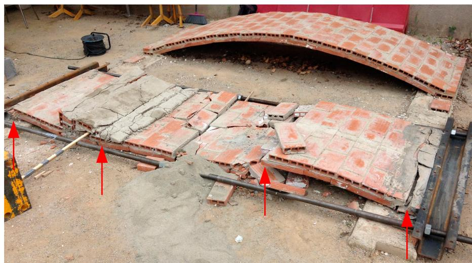
**Figure 8.** First vault collapsed. Red arrows show the identified hinges.
