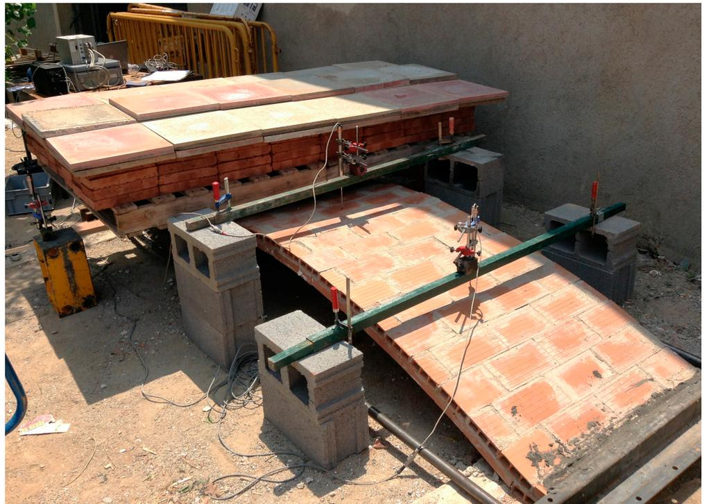
**Figure 9.** Load test on the second vault.
