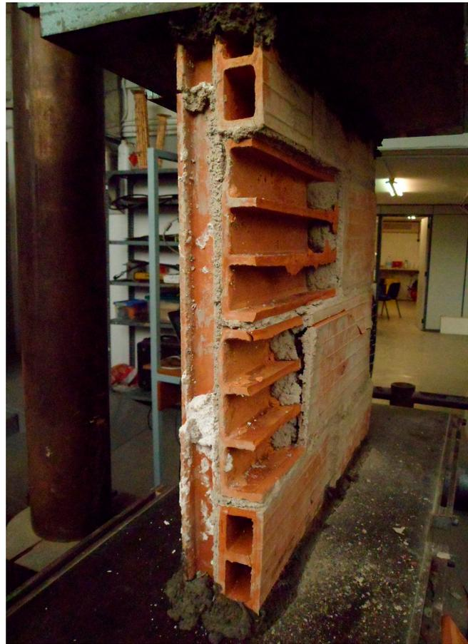
**Figure 1.** Compression test on vault specimens.
