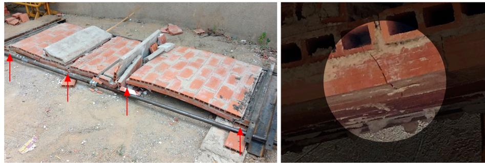
**Figure 11.** Load test on the second vault: (left) end of testing with red arrows showing the identified hinges; and (right) crack during the load test (12.5 kN).
