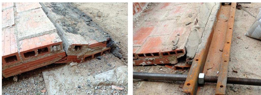
**Figure 13.** Details of the damage at the supports: (left) hinge before the support; and (right) hinge at the support.
