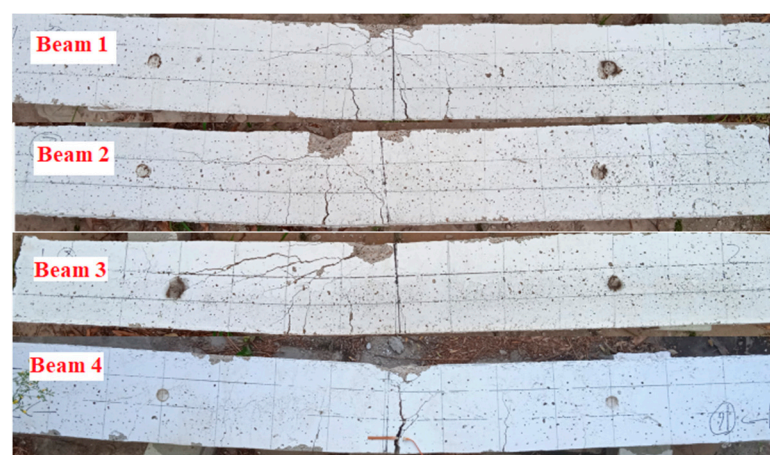
Figure 6. Destruction of beams in the experiments.
