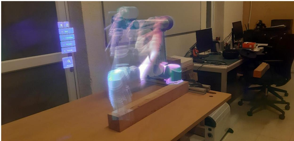
**Figure 18.** Geometry representing the robot's full range of motion at a given instruction, displayed through the mixed reality headset.
