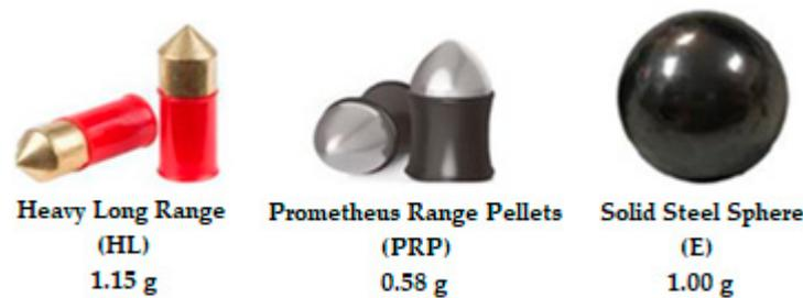
**Figure 4.** Different fragments used for the impact tests.
