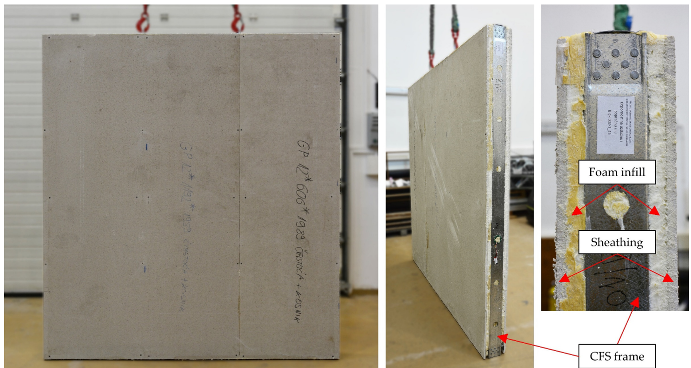
Figure 4. CFS-PU composite wall panel specimen with sheathings and PU foam filling.
