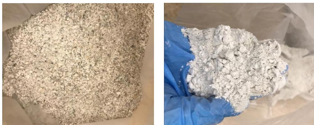
**Figure 4.** Grinding oyster shell to create aggregate (0–4 mm) and powder (150  $\mu\text{m}$ ).
