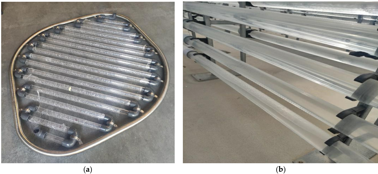
Figure 5. PBR Solar receptors: (a) PBR leaf-like structure (b) Acrylic tubes of PBR façade. Photos from prototypes.
