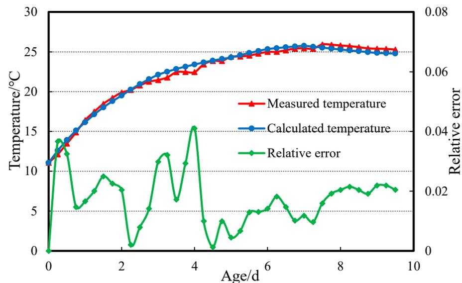
**Figure 10.** Comparison curve and relative errors between measured and calculated temperatures.
