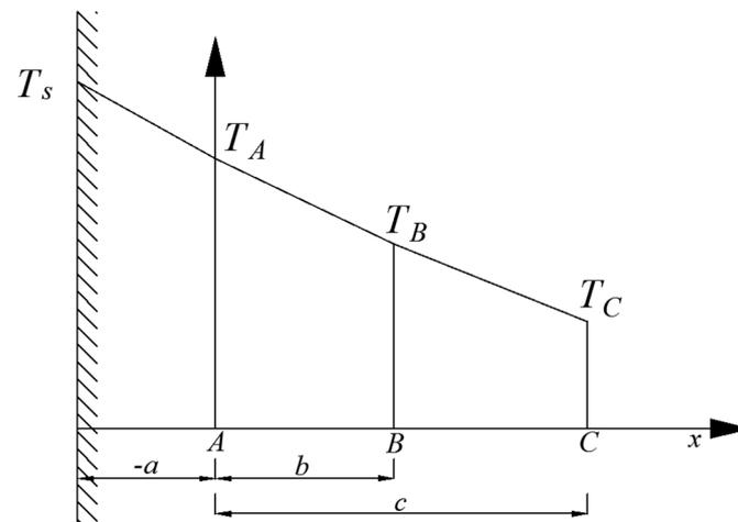
**Figure 3.** Surface temperature distribution of concrete.
