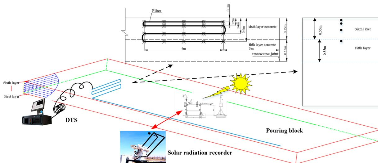
Figure 5. Schematic diagram of the temperature and solar radiant monitoring test plan.
