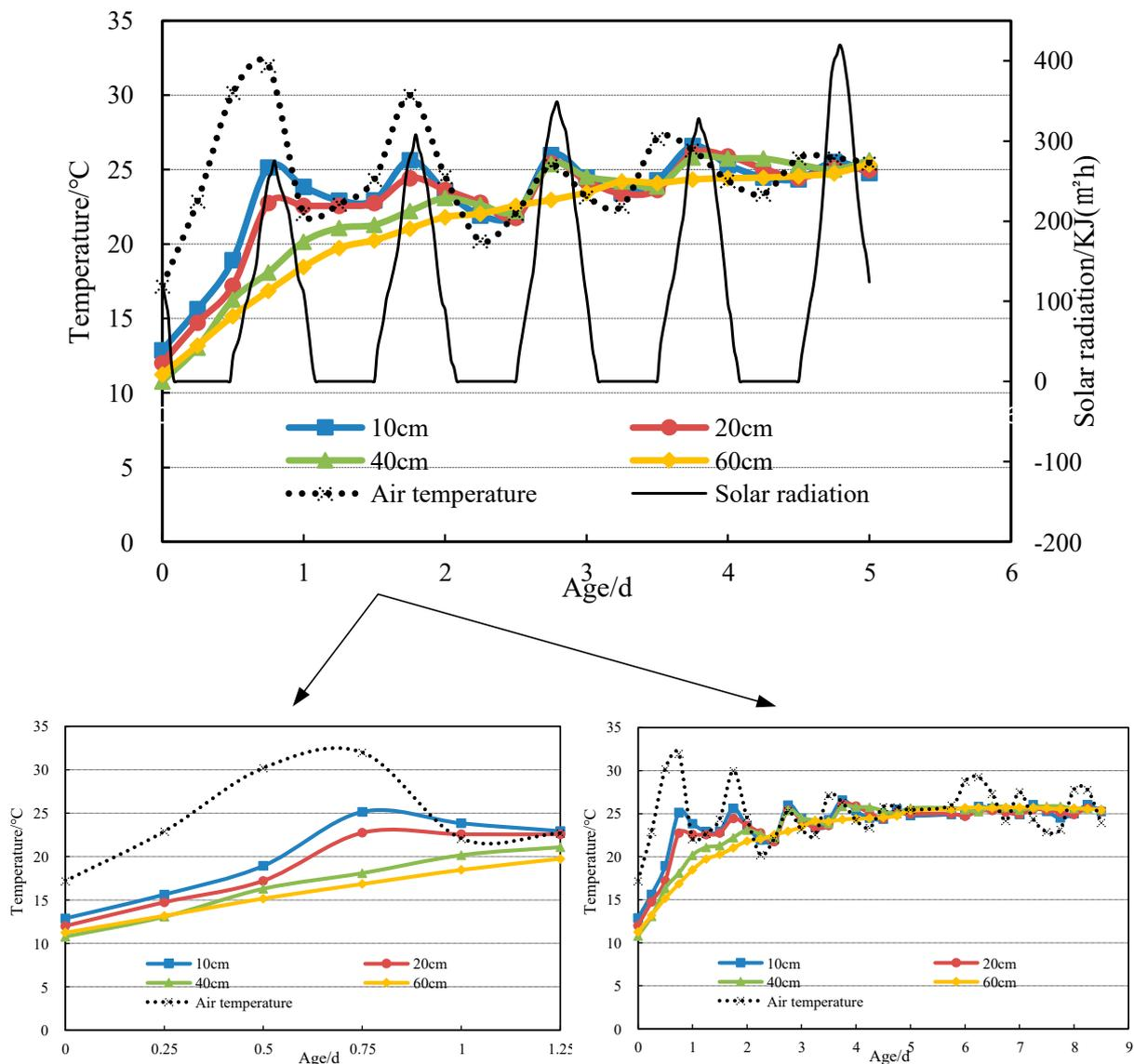
**Figure 7.** The temperature measurement curve of the typical measuring point fiber at different depths from the top surface of the pouring block and the monitoring of the solar radiation intensity.
