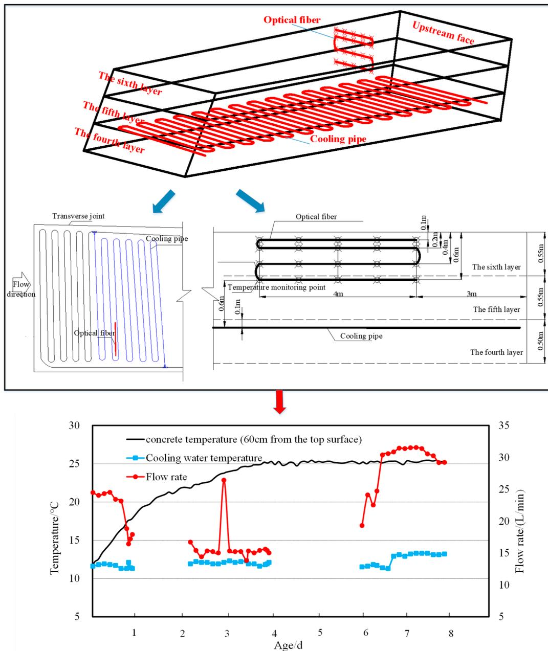
**Figure 8.** Cooling water pipe layout and cooling water parameters.
