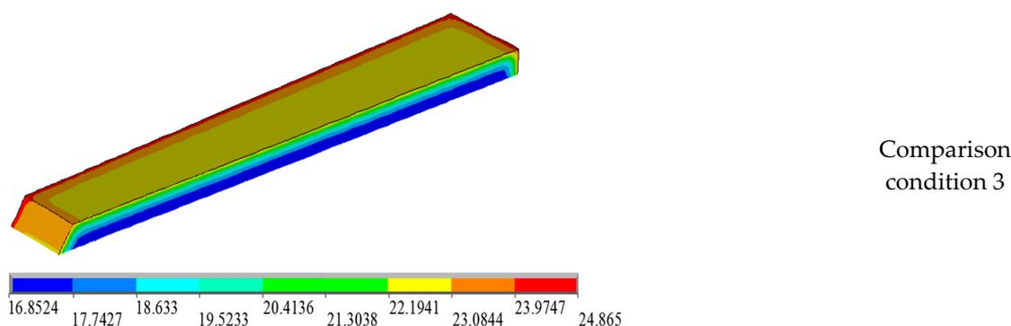
**Figure 14.** Temperature distribution cloud map of pouring blocks along the river center under the basic conditions and comparison conditions 1–3 (A and B are the same two parts of the calculation model divided into two parts).
