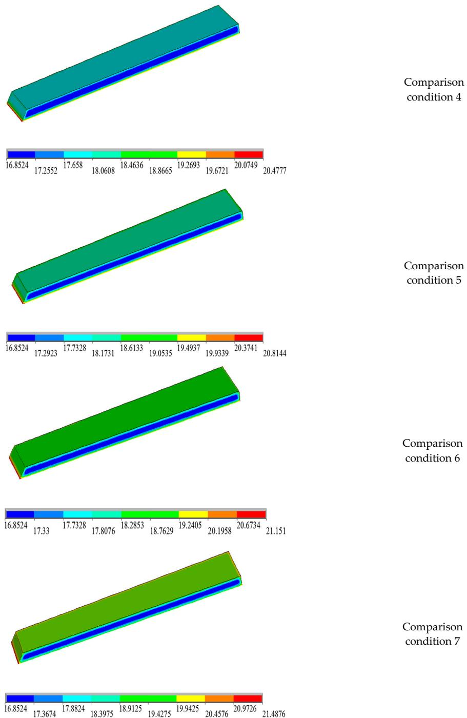
**Figure 17.** Temperature distribution cloud map of pouring blocks along the river center under basic conditions and comparison conditions 4–7.
