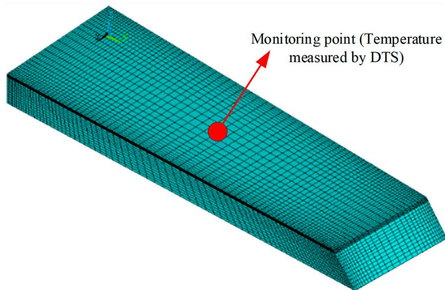
**Figure 9.** Finite element model of a typical concrete block.
