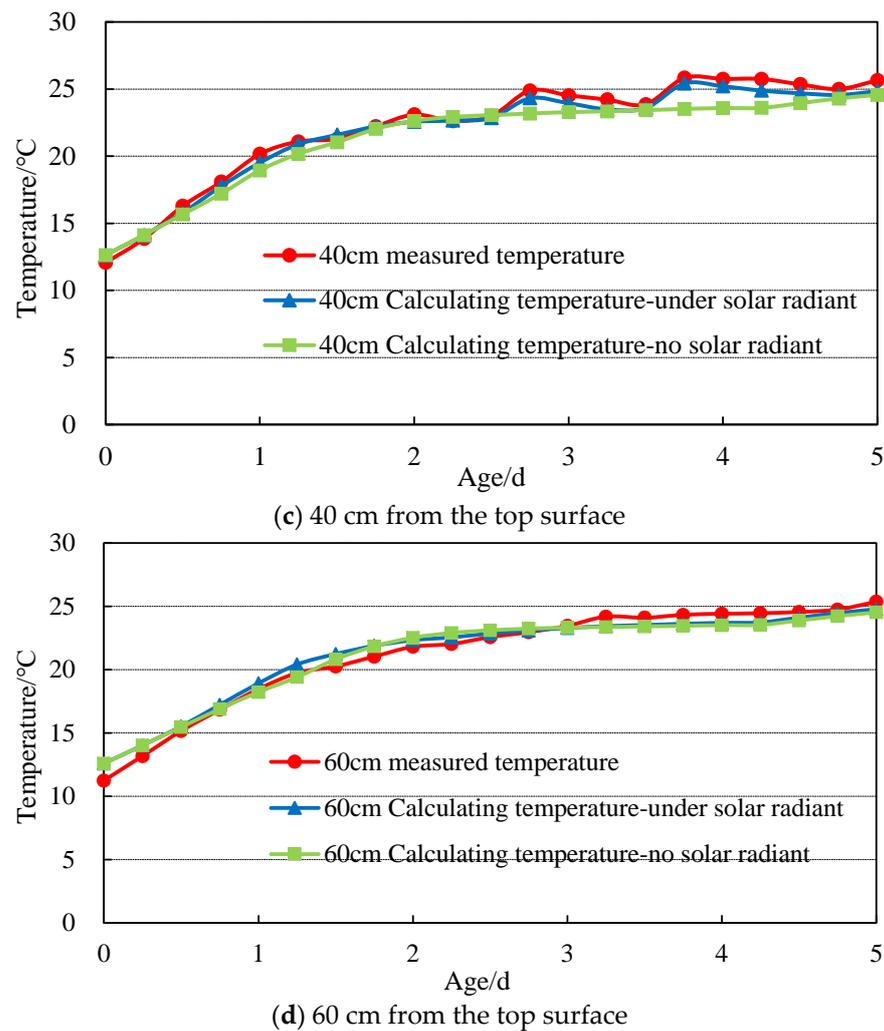
**Figure 11.** Comparison between calculated and measured temperatures at different depths from the surface (condition 1 and condition 2).
