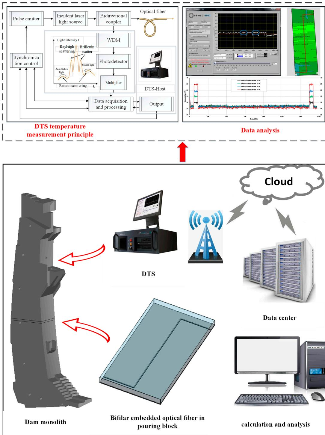
**Figure 2.** Schematic diagram of the bifilar embedded technique of optical fiber based on DTS and the temperature monitoring principle of DTS.
