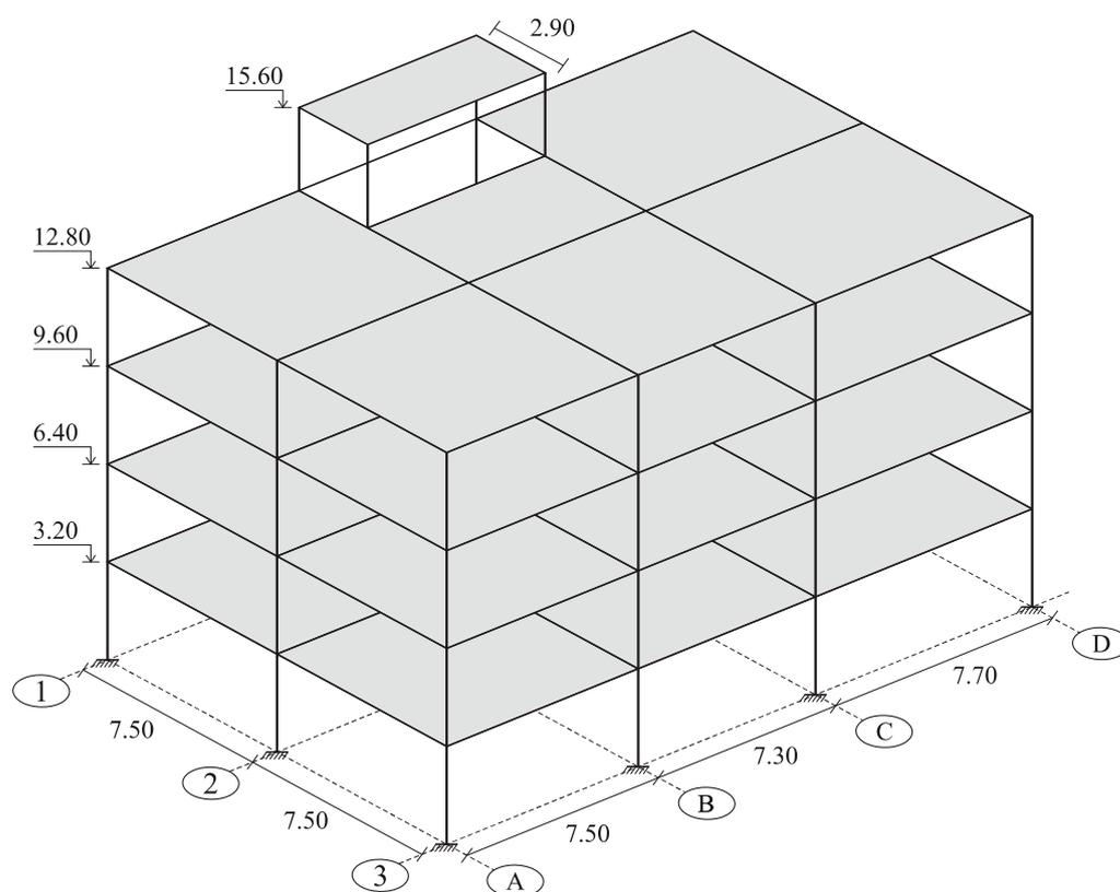
**Figure 1.** A 3D schematic view of the structures (dimensions are in meters).
