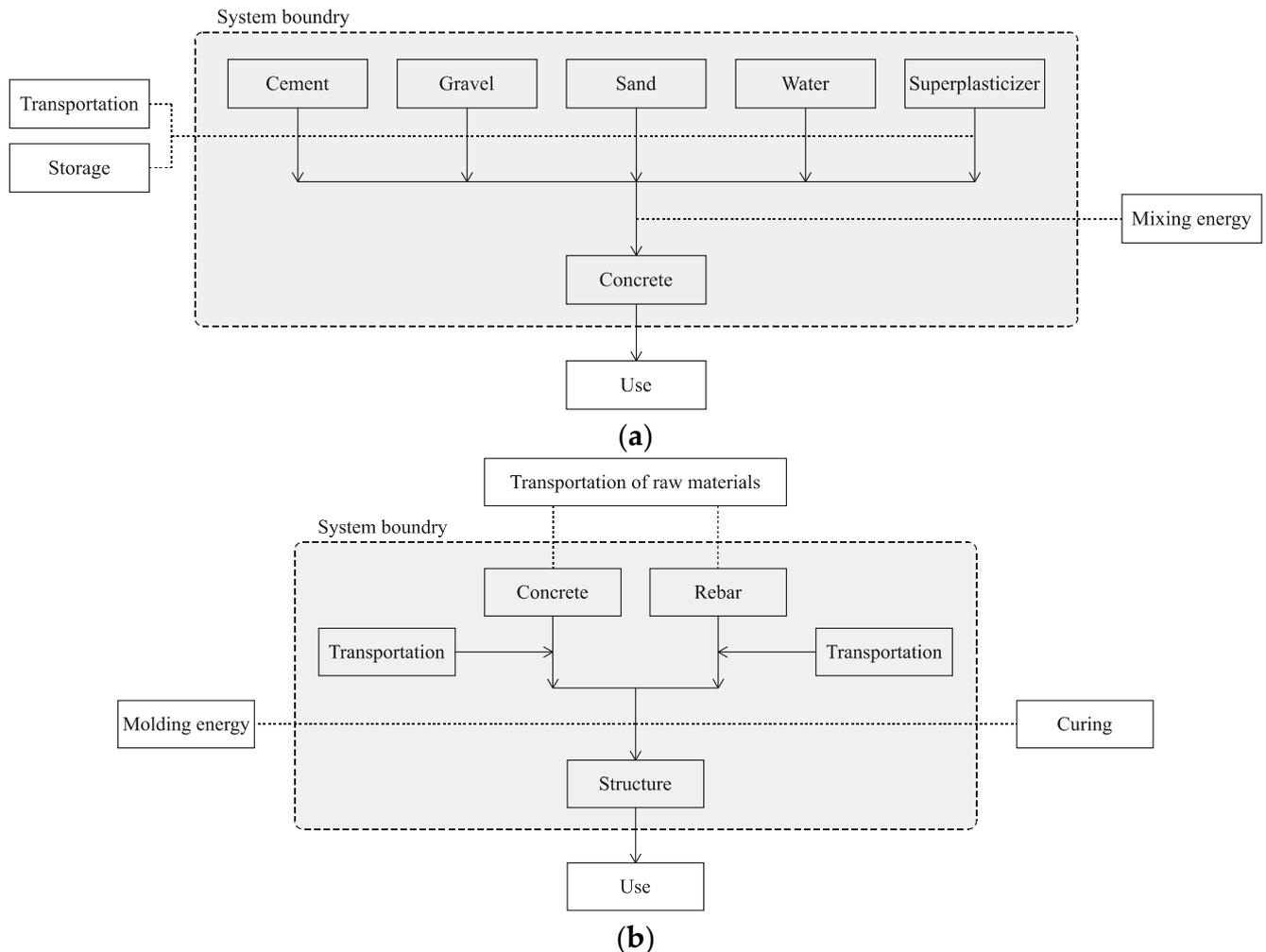
**Figure 2.** The considered system boundaries for the conducted LCA of (a) concrete production ( $1 \text{ m}^3$ ), (b) structure production.
