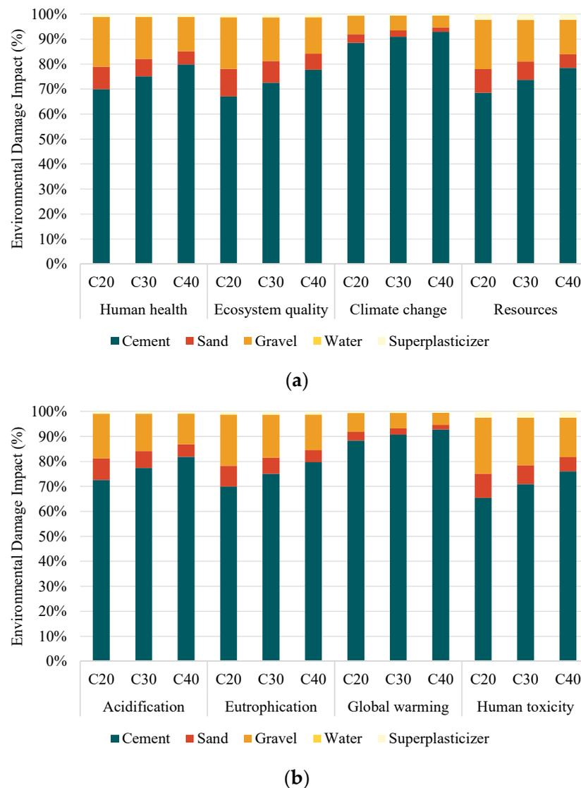
**Figure 3.** LCA results for different concrete mix design parameters based on the (a) IMPACT 2002+, (b) CML baseline 2000.
