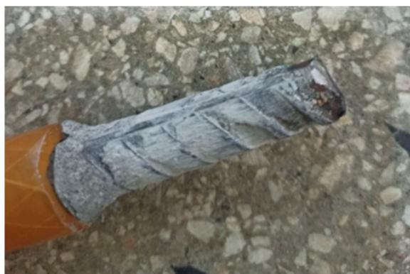
**Figure 31.** Effect of shear stresses generated between bar ribs and concrete at the bond interface.
