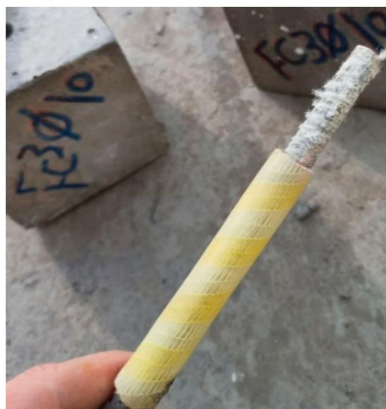
**Figure 32.** Peel off and eroding of the layer covering the GFRP bar during the pull-out test.
