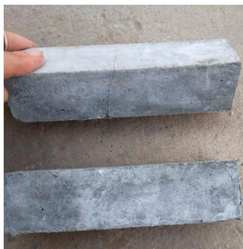
**Figure 9.** FC specimen after flexural test.
