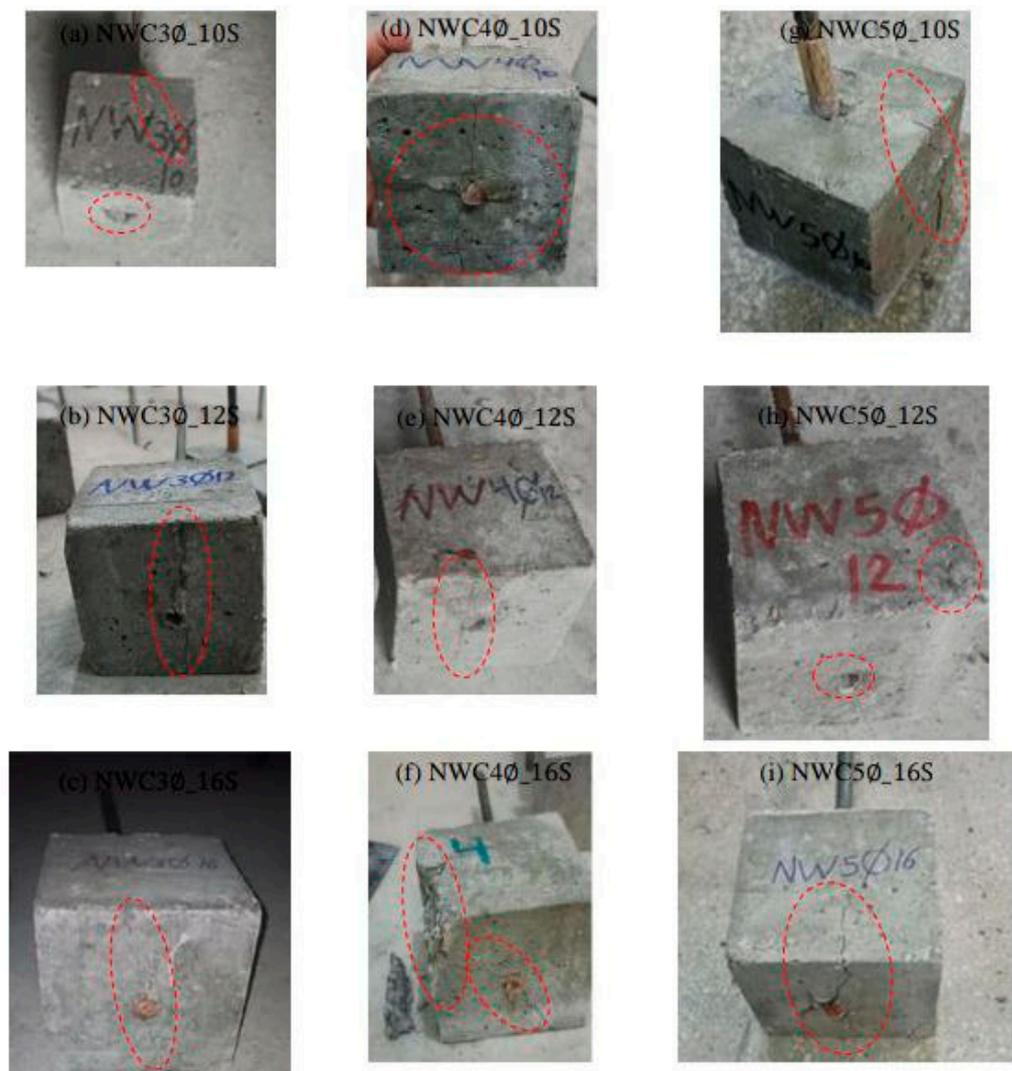
**Figure 27.** Failure patterns of NWC reinforced with ribbed steel bars.
