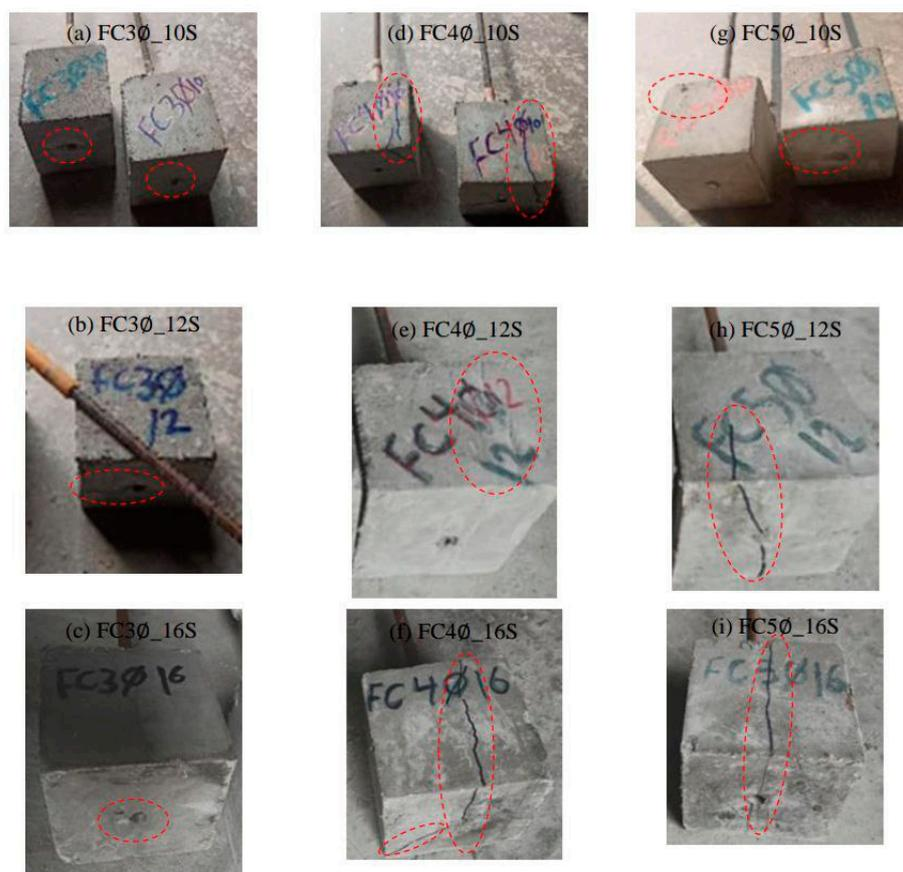
**Figure 13.** Failure patterns of FC reinforced with ribbed steel bars.
