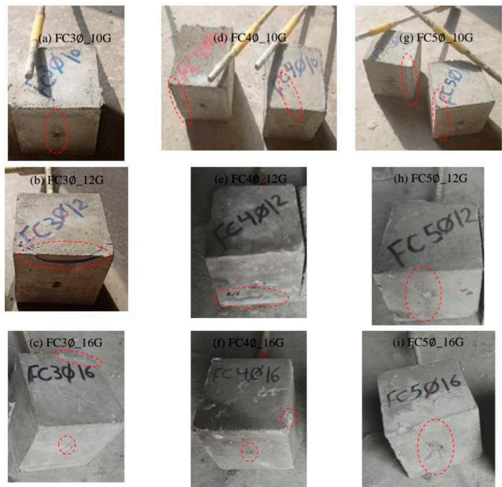
**Figure 20.** Failure patterns of FC reinforced with sand-coated GFRP bars.
