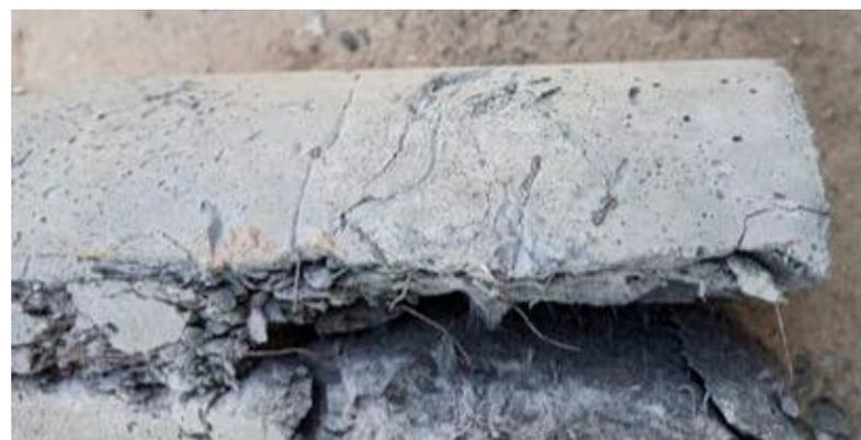
**Figure 8.** Splitting failure of FC.
