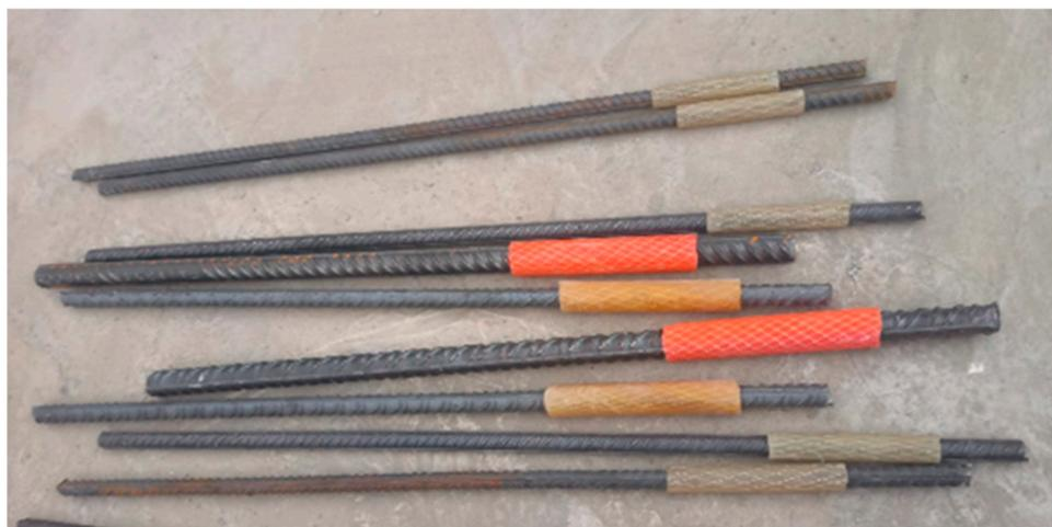
**Figure 4.** The unbonded lengths covered with plastic hollow tube.
