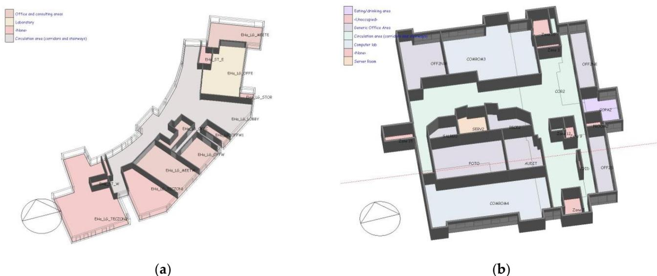
**Figure 2.** Example of thermal zones: (a) GB; (b) non-GB.
