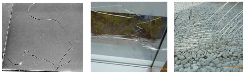
**Figure 6.** Example of glass panes with cracks due to climatic-induced thermal shock (figures reproduced from [60,121] with permission from Elsevier©, copyright license agreement n. 5507161319840, March 2023).
