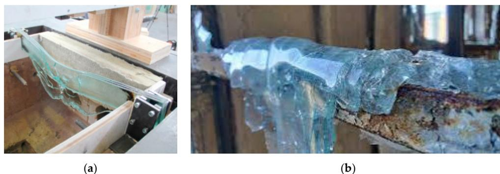
**Figure 7.** Example of collapse configuration for glass under fire: (a) triple-laminated glass beam in bending setup (figure reproduced from [67] with permission from Elsevier©, copyright license agreement n. 5507161319839, March 2023) and (b) details of glass softening in the frame region.
