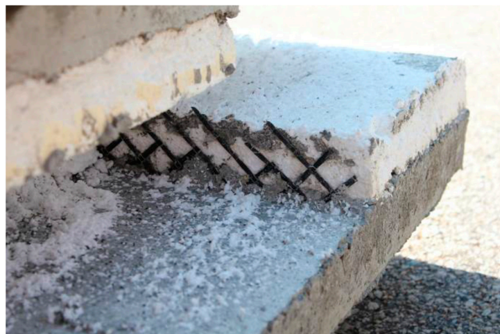
Figure 21. View of ruptured and pulled-out grid.
