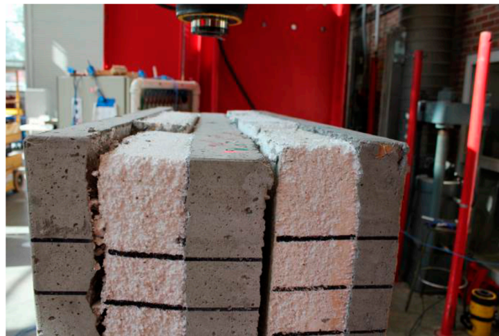
Figure 18. View of a typical failure mode showing shear between wythes.
