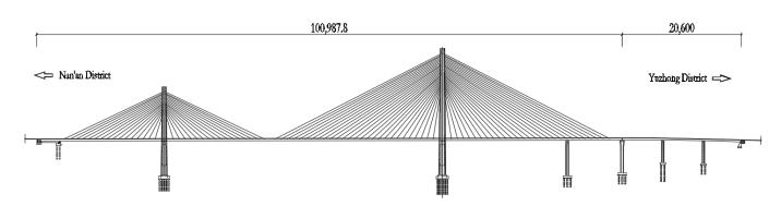
Figure 1. The bridge type layout of Nanjimen Yangtze River Track Special Bridge (unit: mm).
