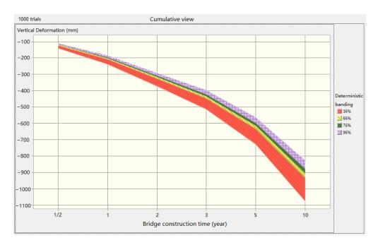
Figure 8. Vertical deformation predicted interval at different confidence levels.
