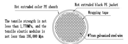
Figure 4. Cross-sectional view of the cable.
