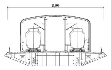
Figure 2. Cross-sectional view of the main beam (unit: mm).
