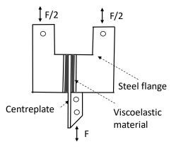
Figure 15. Improvement of Viscous Damper.
