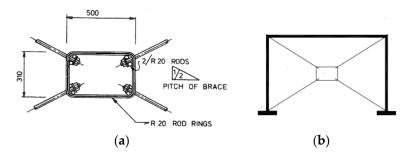
**Figure 8.** Premier metallic damper. (a) description of the rectangular metallic damper, (b) one story frame with the metallic damper.
