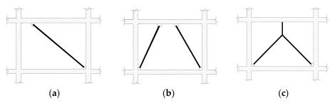
**Figure 2.** Several schematic models with eccentric bracing systems: (a) single diagonal bracing with eccentricity, (b) double diagonal bracing with eccentricity, (c)  $\Lambda$  bracing with eccentricity.
