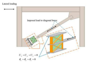
Figure 10. A new MD that improves the behavior of the shear dampers [129].
