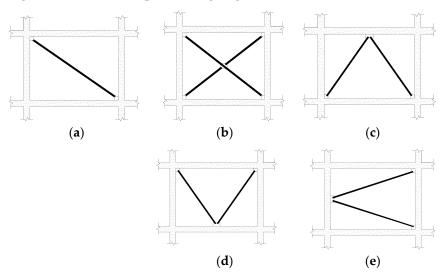
**Figure 1.** Concentrically Braced Frames: (a) single diagonal bracing, (b) cross bracing, (c)  $\Lambda$  bracing (chevron), (d) V bracing (chevron), (e) K bracing.
