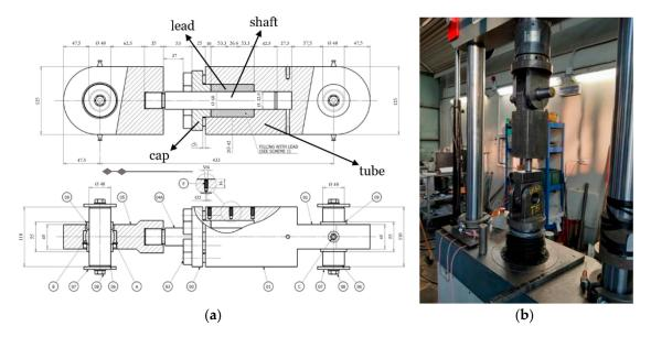
**Figure 12.** PS-LED damper proposed by Quaglini et al. able to reduce the costs of production: (a) description of the damper, (b) experimental set-up [160].
