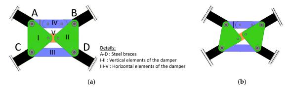
**Figure 6.** Construction of the improved Pall friction damper proposed by Papadopoulos, (a) inactive damper, (b) activation of the damper.
