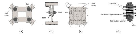
**Figure 4.** Improvement of PFD proposed by Anagnostides et al.: 1. three plates damper with high-strength bolts (a) longitudinal section, (b) cross-section. 2. twelve friction joints incorporating frictional washers (c) longitudinal section, (d) cross-section.
