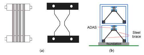
Figure 9. (a) Description of ADAS damper, (b) two story frame with ADAS damper.
