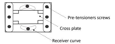
Figure 3. Pall friction damper.
