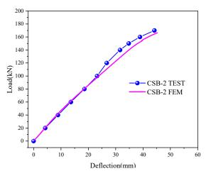
Figure 13. The overhanging end deflection of test value and FEM calculated value of CSB-2.
