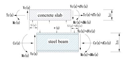
Figure 9. Internal force distribution in a microsegment of the beam.
