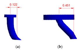
**Figure 15.** Displacement difference between the top and bottom of the studs at Section 2-2 (mm). (a) CSB-1. (b) CSB-2.
