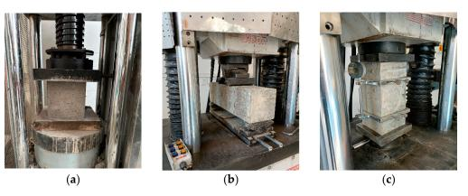
**Figure 2.** Mechanical property test of concrete. (**a**) Cube compressive strength. (**b**) Bending and tensile strength. (**c**) Elastic Modulus.
