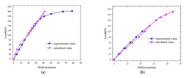
Figure 10. Comparison of calculated and tested deflection of the overhanging end. (a) CSB-1. (b) CSB-2.
