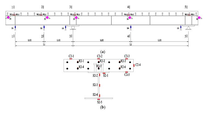
**Figure 4.** Instrumentation arrangement on a specimen. (**a**) Gauges of deflection, slip, and strain of studs. (**b**) Strain gauges of concrete, steel beam, and steel bar at Section 2-2.
