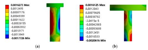
**Figure 14.** Axial strain of the studs at Section 2-2 (με). (a) CSB-1. (b) CSB-2.
