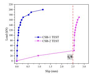
Figure 6. Load-slip curves.
