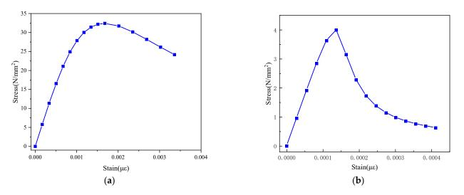
**Figure 11.** Stress-strain curve of concrete. (**a**) The compressive stress-strain curve. (**b**) The tensile stress-strain curve.
