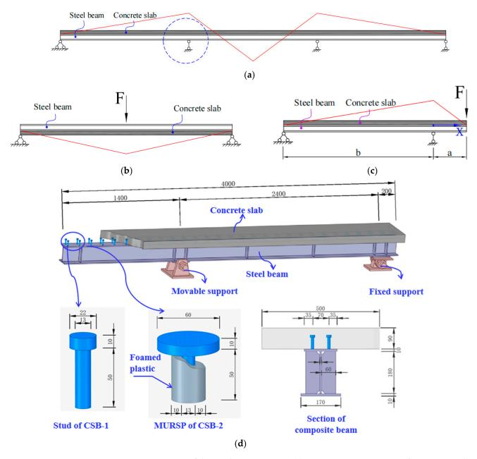
**Figure 1.** Structure of the overhanging SCCBs. (**a**) Negative moment region of a continuous beam. (**b**) Overturned simply supported beam. (**c**) Overhanging beam. (**d**) Dimensions of the test specimen.
