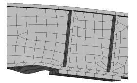
Figure 12. Buckling of the steel beam of CSB-1.
