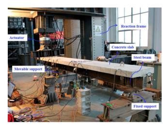
Figure 3. Experimental setup.
