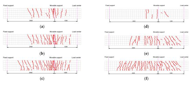
Figure 5. Crack distribution. (a) CSB-1 60 kN. (b) CSB-1 100 kN. (c) CSB-1 170 kN. (d) CSB-2 60 kN. (e) CSB-2 100 kN. (f) CSB-2 170 kN.
