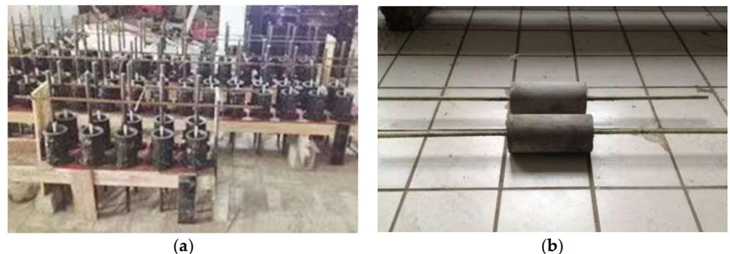
**Figure 2.** Fabrication of concrete specimens with GFRP bars: (a) Molds secured in place; (b) Concrete specimens with GFRP bars.
