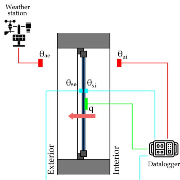
**Figure 4.** The principle of experimental measurement in the pavilion laboratory.
