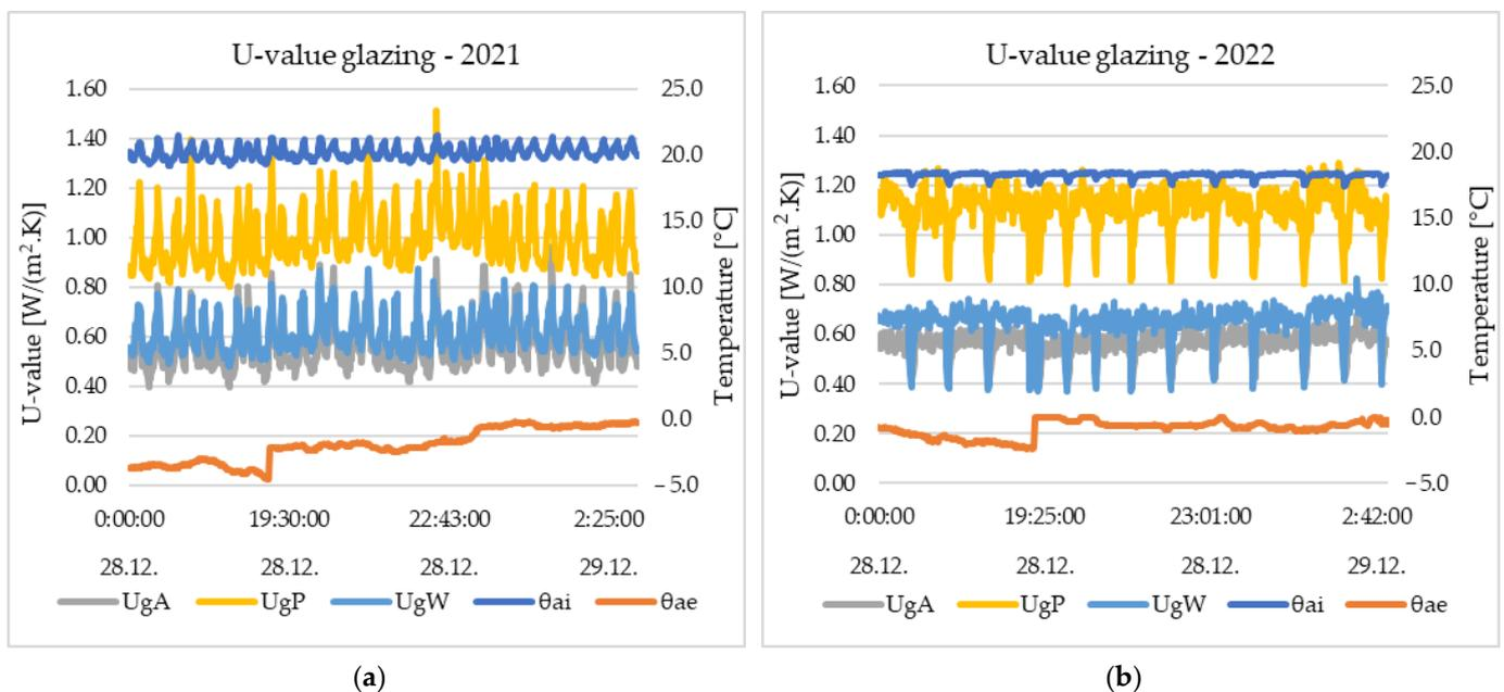
**Figure 8.** U-value glazing of all three window constructions on the selected date: (a) 2021; (b) 2022.
