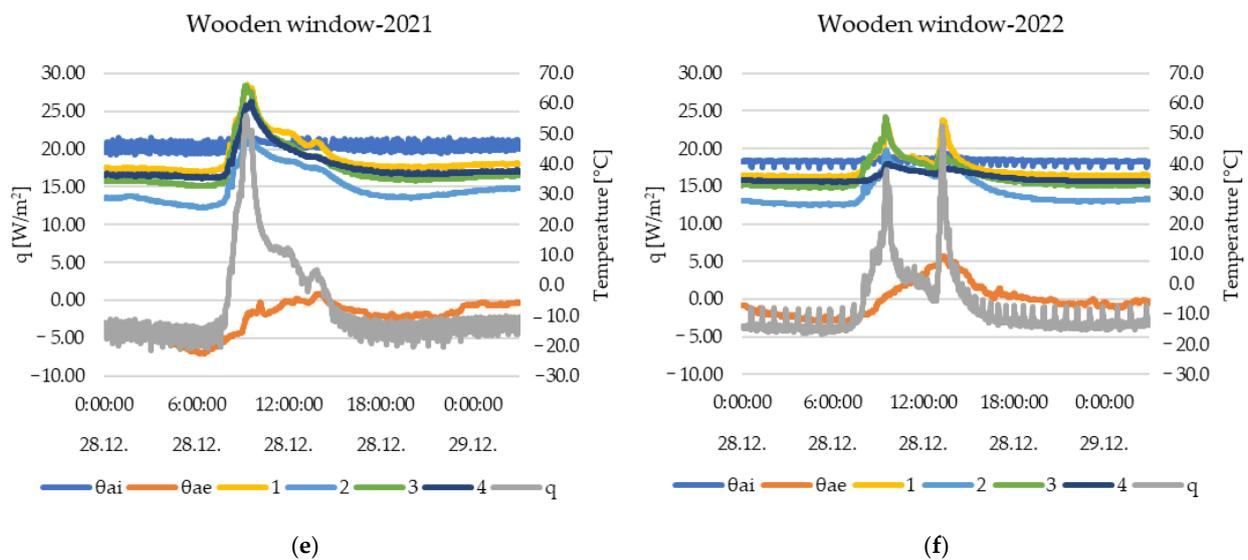
**Figure 7.** Measured data on all three window constructions on the selected date: (a) Aluminum window in 2021; (b) Aluminum window in 2022; (c) PVC window in 2021; (d) PVC window in 2022; (e) Wooden window in 2021; (f) Wooden window in 2022.
