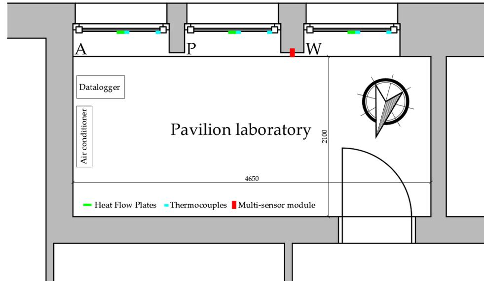
Figure 3. Plan of the pavilion laboratory.
