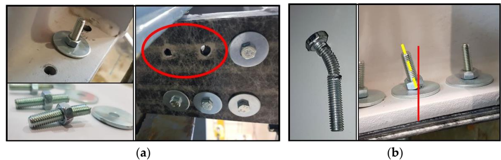
Figure 8. (a) Shear fracture of the bolts in U45D35; (b) bending of the bolts in U45D35.
