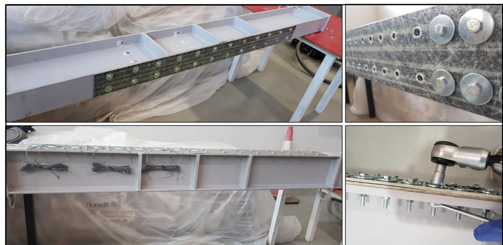
Figure 3. Pictures of fastening the of the HFRP strips to the bottom steel flange.
