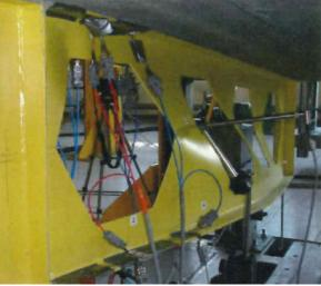
Figure 6. Lateral distortional buckling in steel-concrete composite alveolar beams [58].
