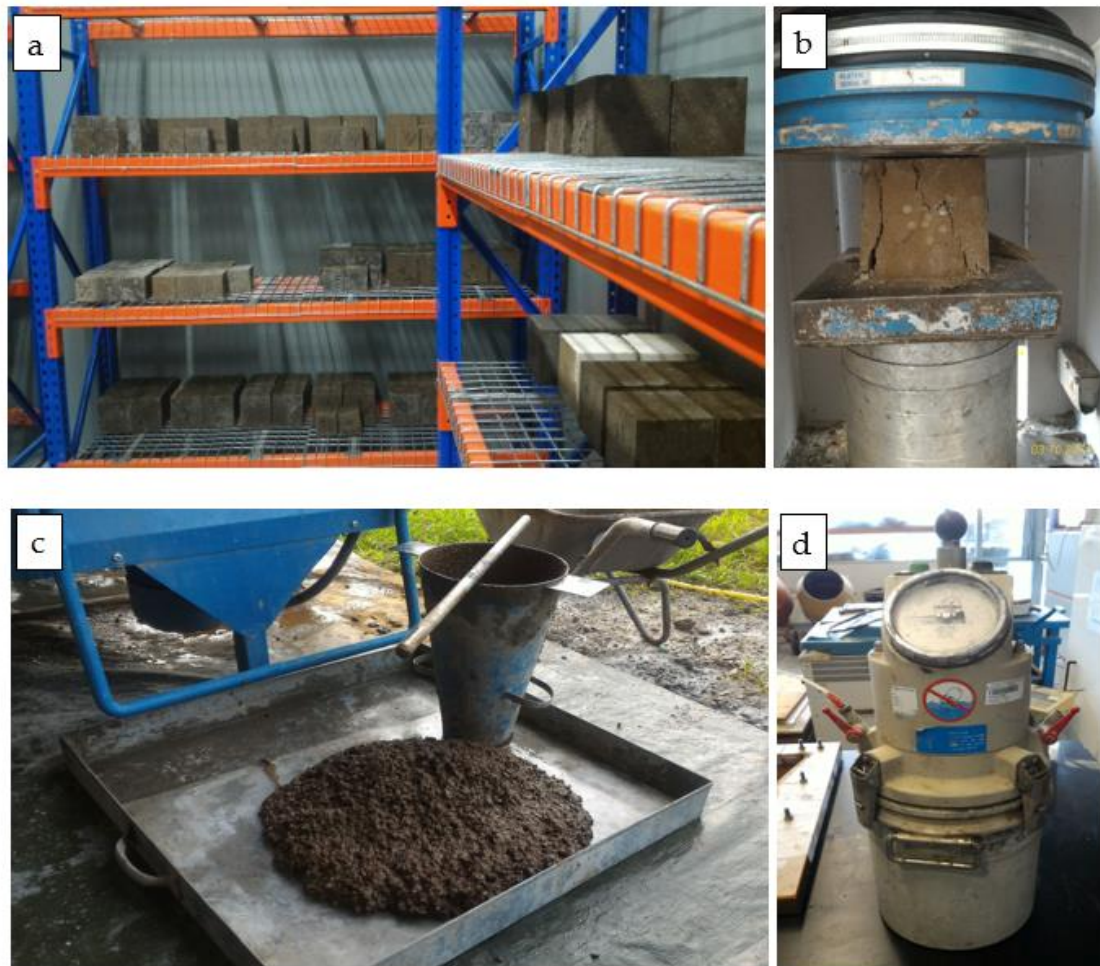
Figure 1. (a) Concrete specimens, (b) loading machine, (c) slump test, and (d) air content apparatus, respectively.
