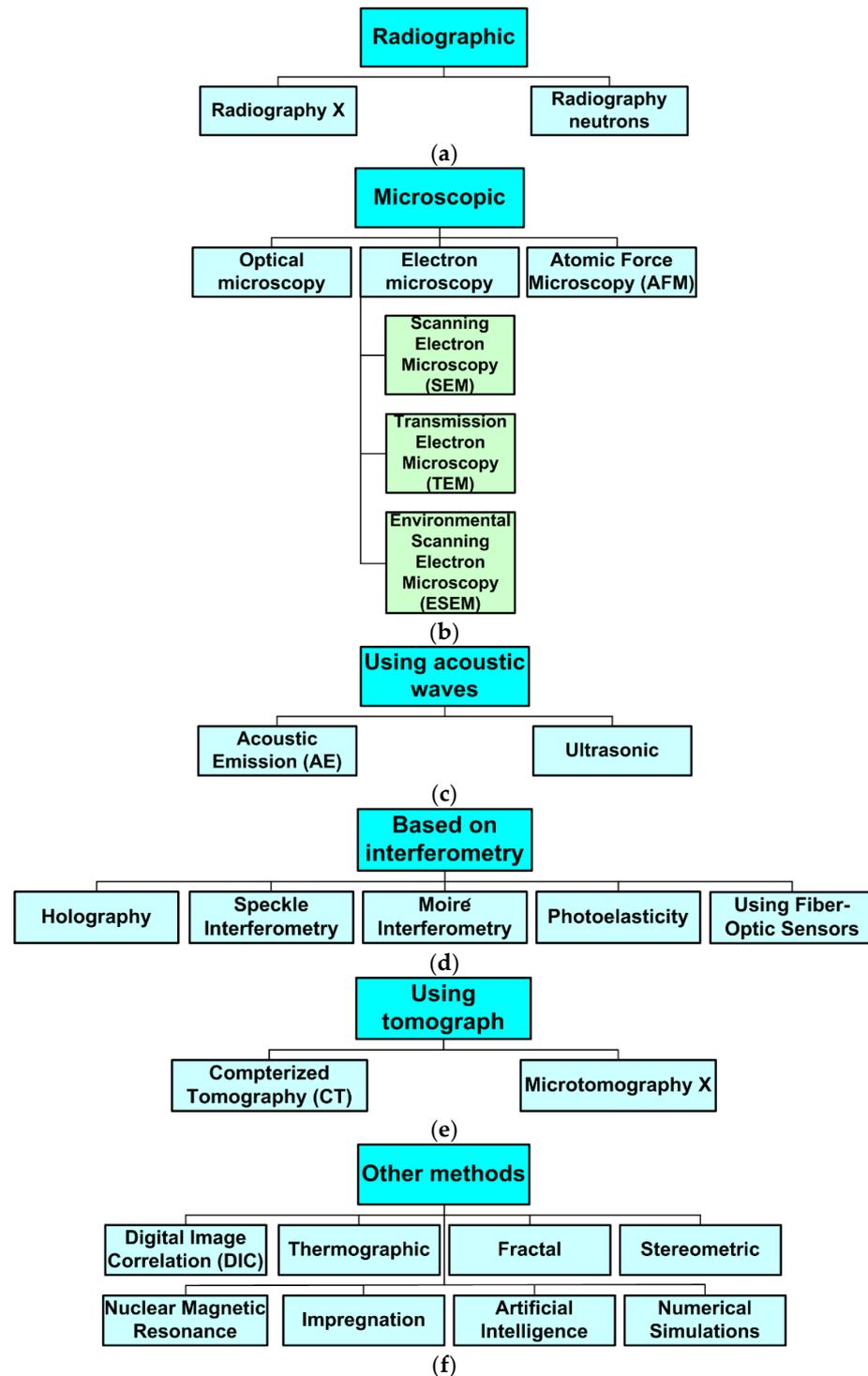
**Figure 10.** The most important methods for the detection and analysis of microcracks and cracks in cement concretes: (a) [185–193], (b) [173,194–204], (c) [204–213], (d) [177,214–217], (e) [179–182] and (f) [218–225].
