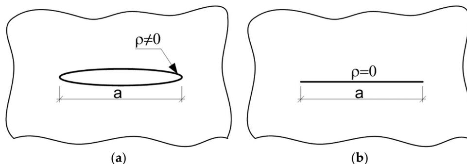
**Figure 1.** Diagrams of material defects in concrete: (a) crack, (b) gap [66–68].
