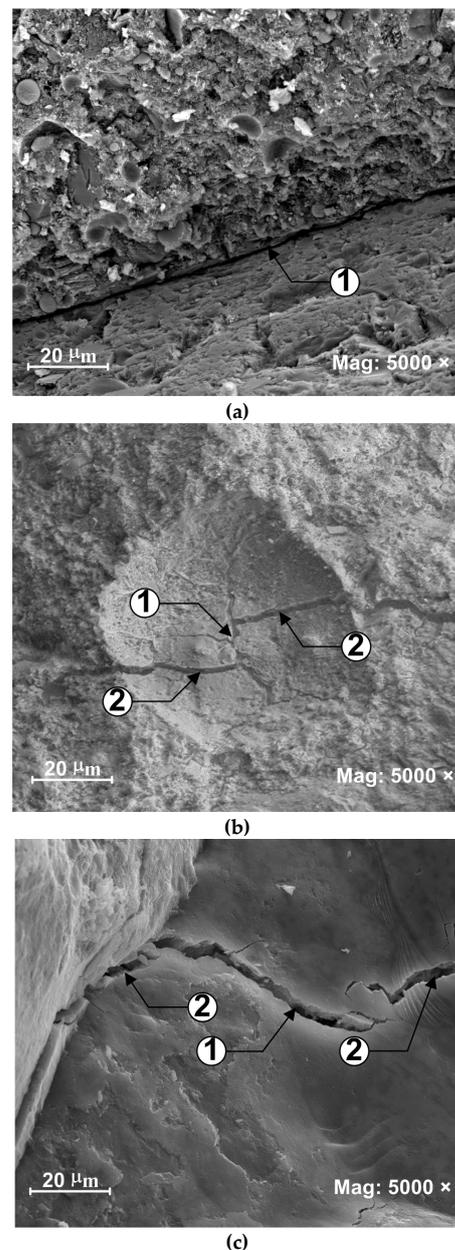
**Figure 9.** Microcracks occurring in concrete structures caused by stresses: (a) tensile stress, (b) shear stress, (c) torsion stress; 1—straight crack, 2—wing.
