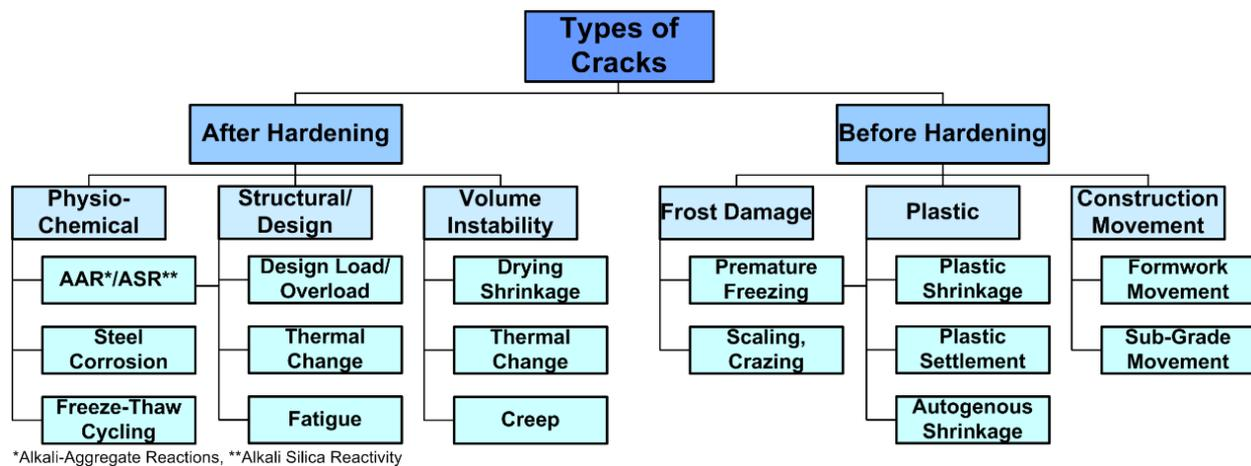
Figure 3. Common causes for cracking in concrete structures (according to [119]).
