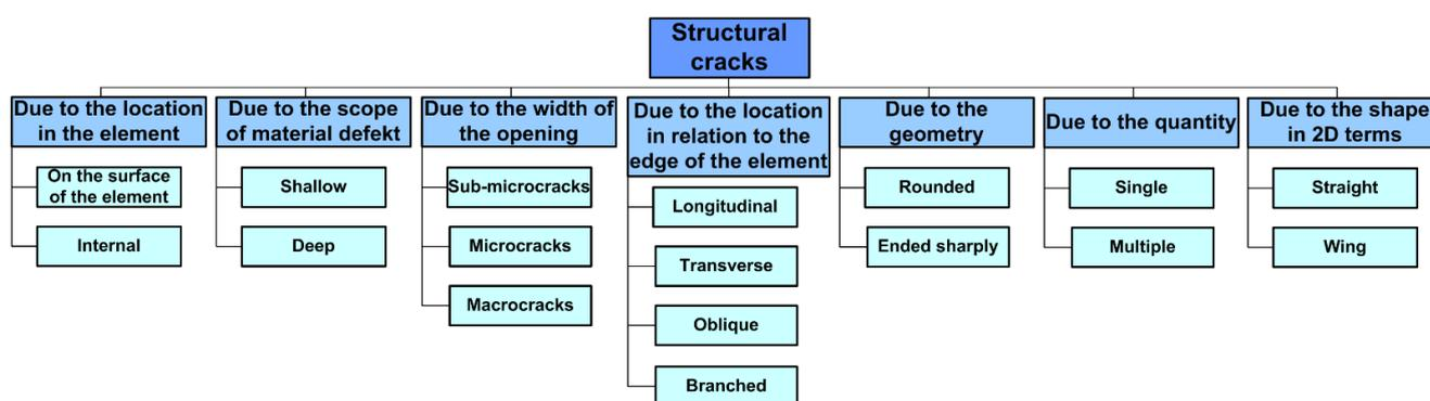
Figure 4. Breakdown of structural cracks in concrete.
