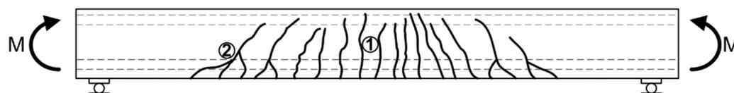
Figure 6. Macrocracks due to bending; 1—single cracks, 2—collective cracks,  $M$ —bending moment.
