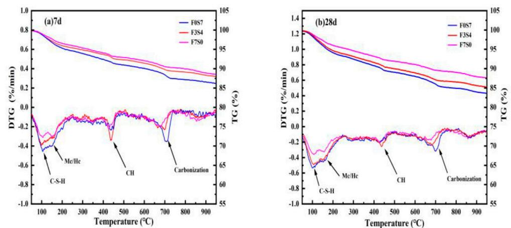
Figure 6. TG–DTG curves of the LCFLS: (a) 7 d; (b) 28 d.
