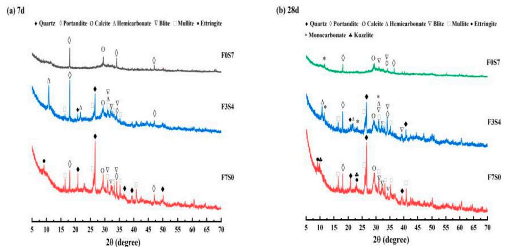
Figure 5. XRD patterns of the LCFLS: (a) 7 d; (b) 28 d.
