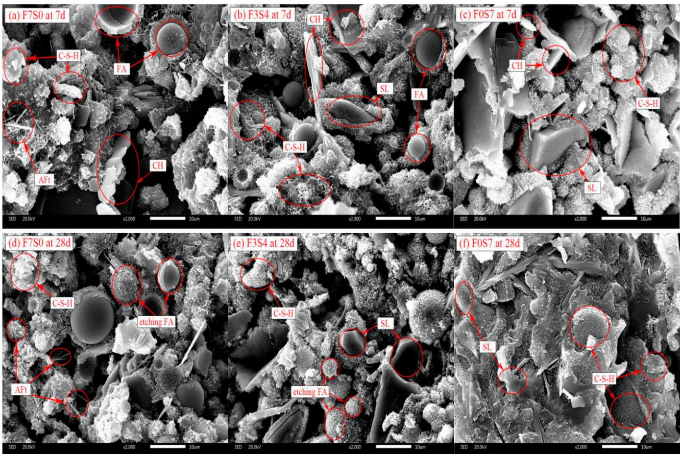
Figure 8. SEM images of the LCFLS at 2000× magnification.
