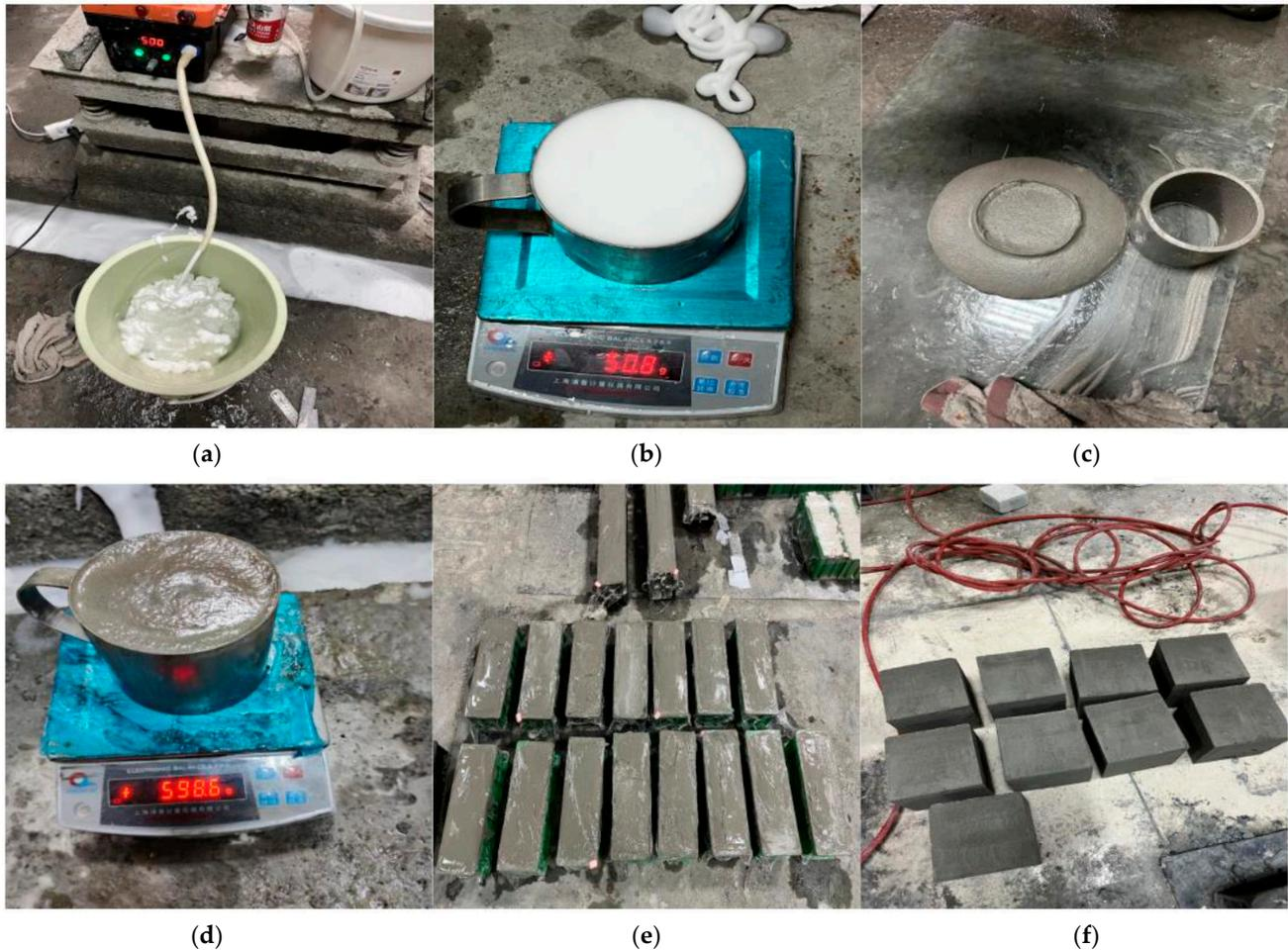
**Figure 1.** Production process of LCFLS: (a,b) foam preparation; (c,d) measurement of flowability and wet density; (e,f) molding and curing.
