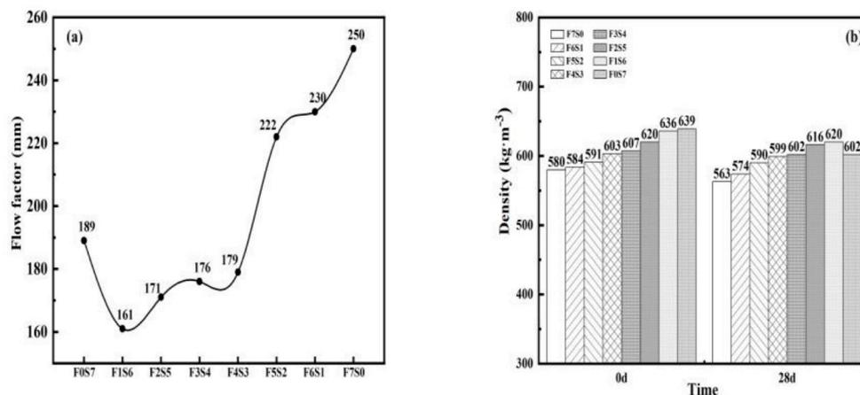
**Figure 2.** Working performance of the LCFLS: (a) flowability; (b) wet density and quasi-dry density.
