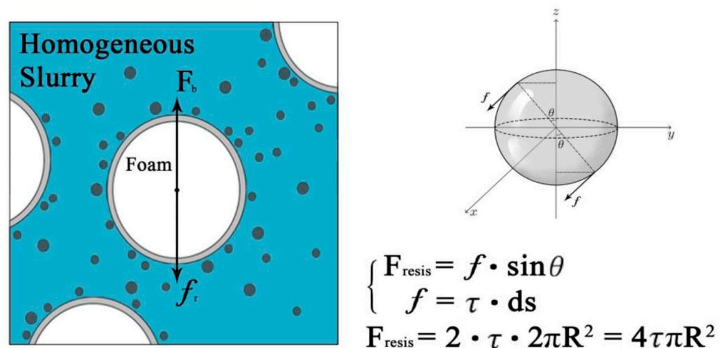
Figure 11. Force analysis of foam in LCFLS.
