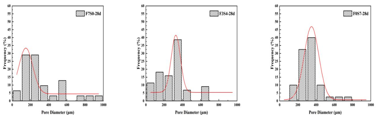
Figure 9. Pore size distributions of LCFLS.
