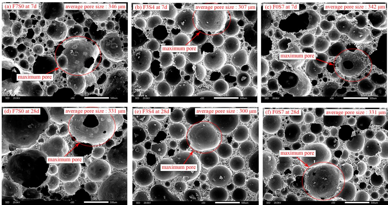
**Figure 7.** SEM images of the LCFLS at 50  $\times$  magnification.
