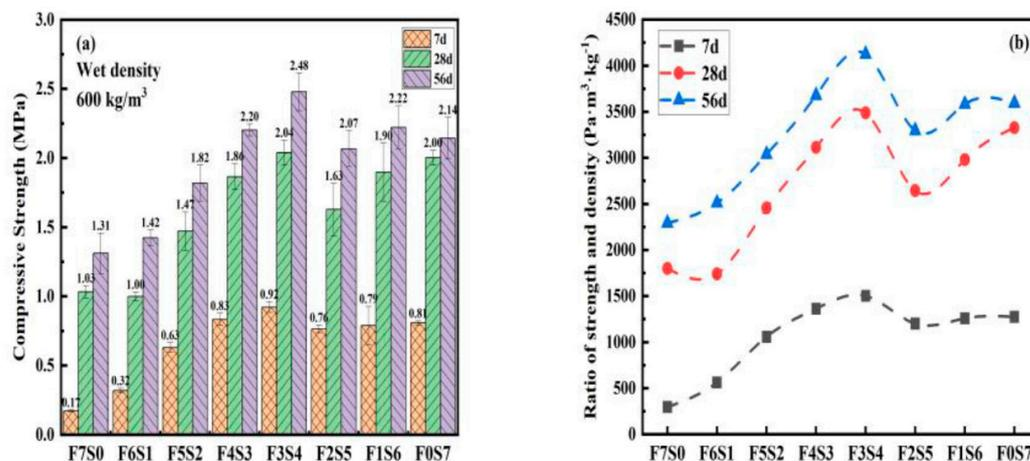
**Figure 4.** Mechanical performance of the LCFLS: (a) compressive strength; (b) ratio of strength and density.
