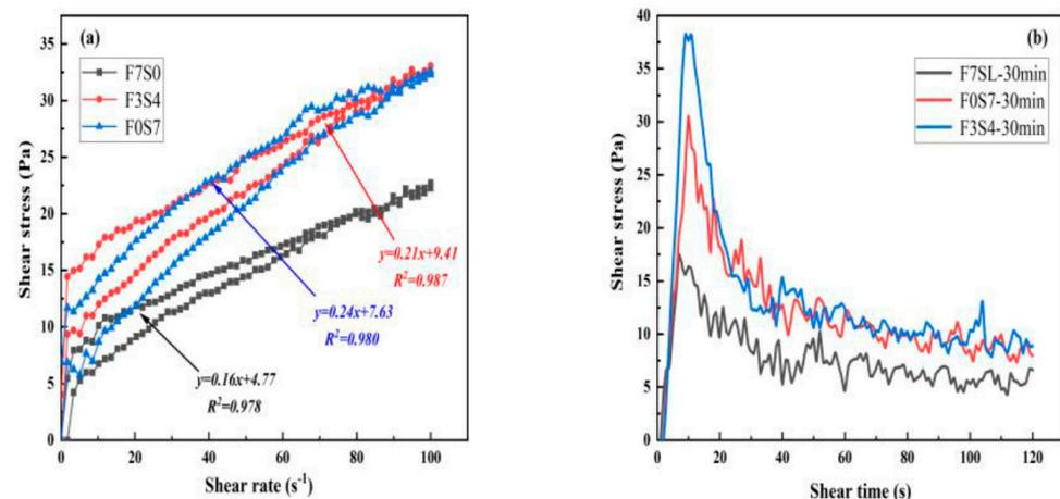
**Figure 3.** Rheological properties of the LCFLS: (a) dynamic yield stress at 0 min; (b) static yield stress at 30 min.
