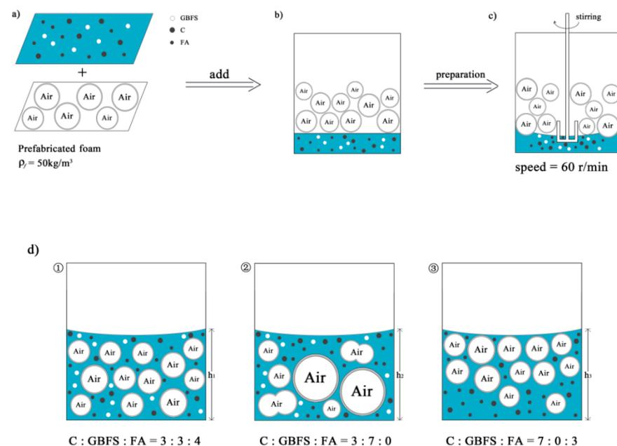
Figure 10. Theoretical mixing process of LCFLS.
