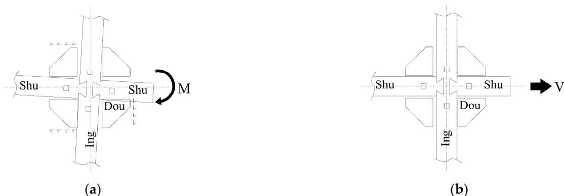
Figure 5. Relative movement of the components in Zuo-Dou joints: (a) horizontal rotation; (b) in-plane shear.
