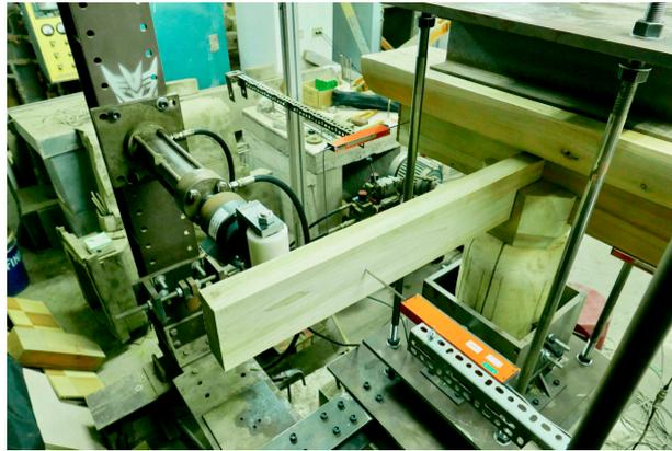
Figure 9. Testing rig and specimen of rotational test.
