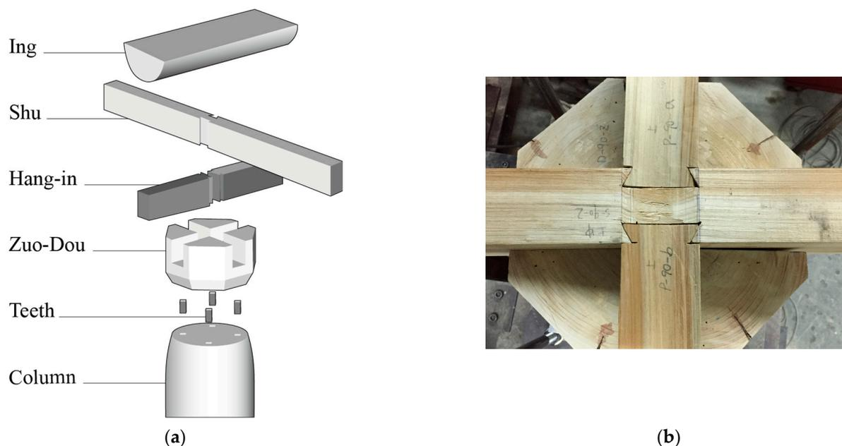
**Figure 3.** Zuo-Dou as beam-to-column joint: (a) connection in the column's top; (b) components on the Zuo-Dou.
