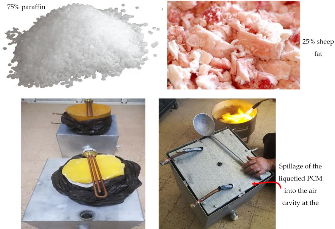
**Figure 5.** Design elements of the storage tanks; the liquefied PCM incorporation in the lateral layers of the storage tank.
