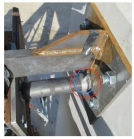
(a) EAC with ICP force sensor 200C20
