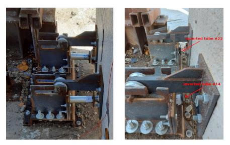
**Figure 10.** Sample panel  $4A - \phi 42 \times 1.5$  mm tubes: before blast (**left**) and after blast test (**right**).
