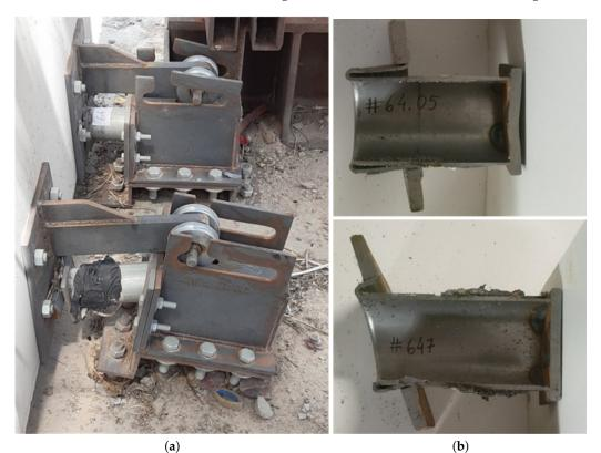
**Figure 12.** Sample panel 2B.(**a**) General view of anchor deformation after blast for connectors #64.05 and #647. (**b**) Longitudinal section: final state of the inversion of  $\phi$ 64 × 2.0 mm tubes.
