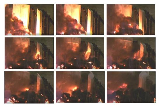
Figure 9. Footage of the blast wave of 60 kg RIODIN Dynamite at 5 m (test #3).
