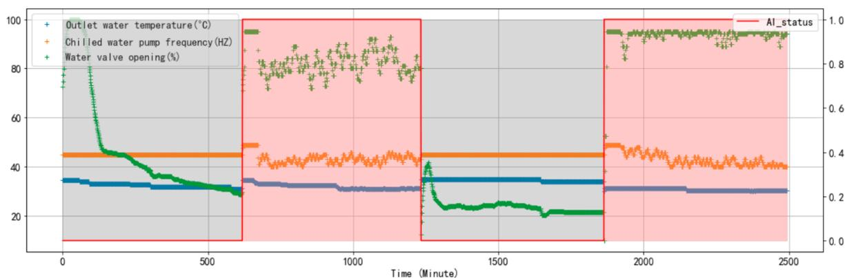
**Figure 11.** Action trends of AB tests (the grey area represents the AI\_status is 0, the red area represents the AI\_status is 1).
