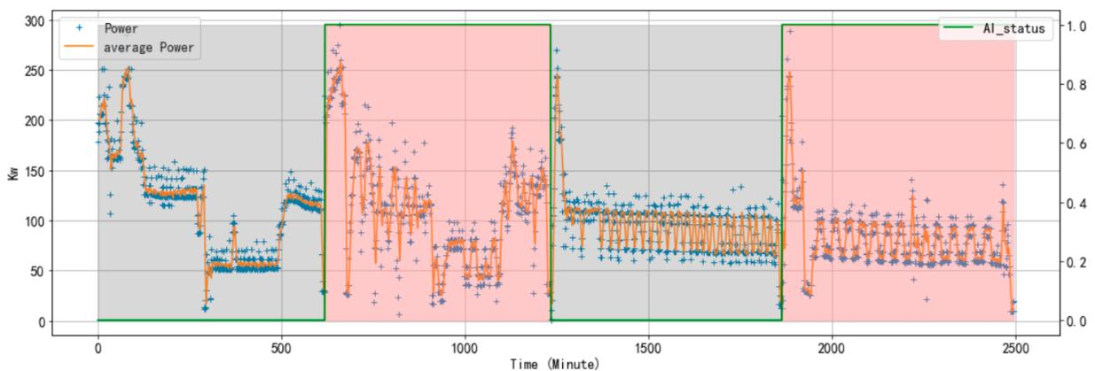
Figure 10. Power trends of AB tests (the grey area represents the AI\_status is 0, the red area represents the AI\_status is 1).
