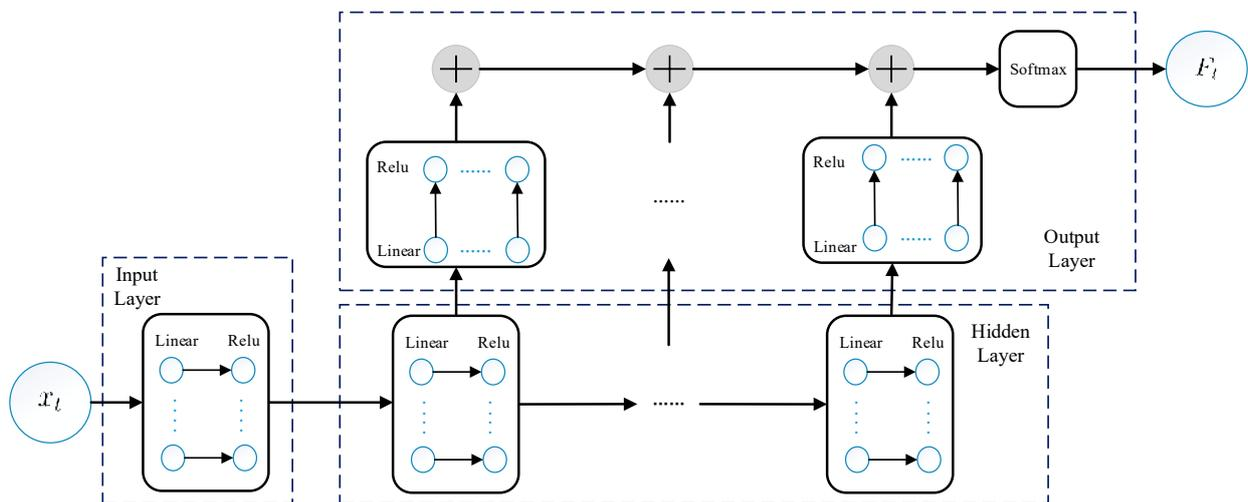
**Figure 4.** The network of the online safety classifier based on residual learning.
