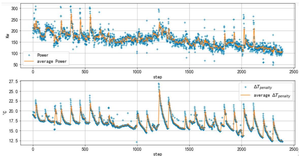
Figure 8. Power consumption and indoor temperature penalty trends of proposed RL algorithm.
