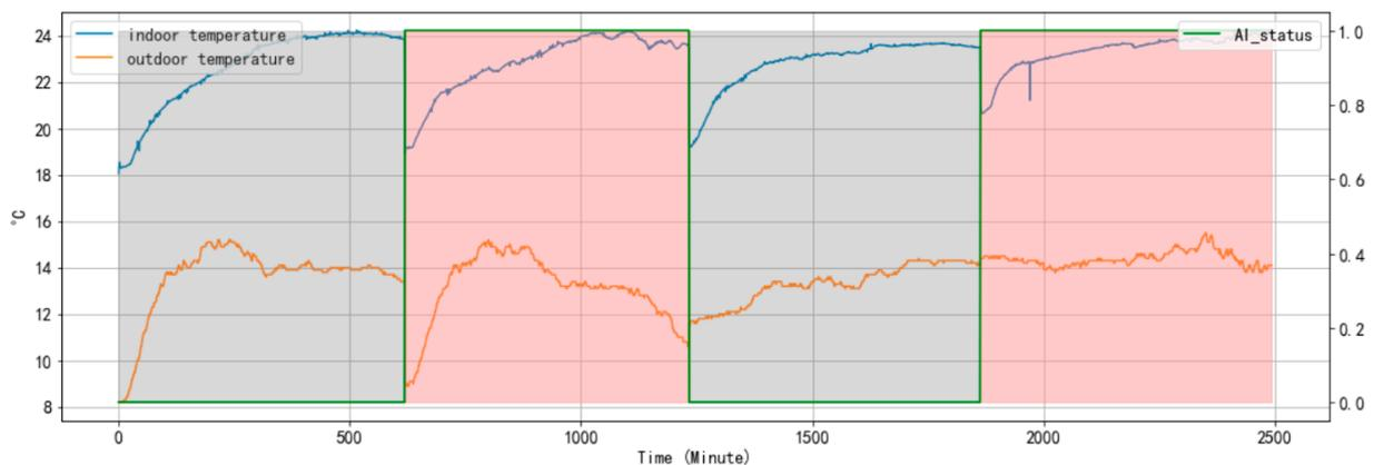
Figure 9. Temperature indoor and outdoor trends of AB tests (the grey area represents the AI\_status is 0, the red area represents the AI\_status is 1).
