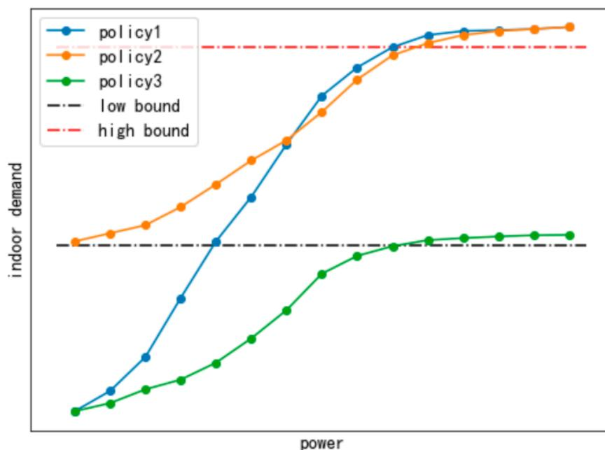
**Figure 2.** Schematic diagram of the corresponding relationship between the consumed power and the indoor demand satisfaction.
