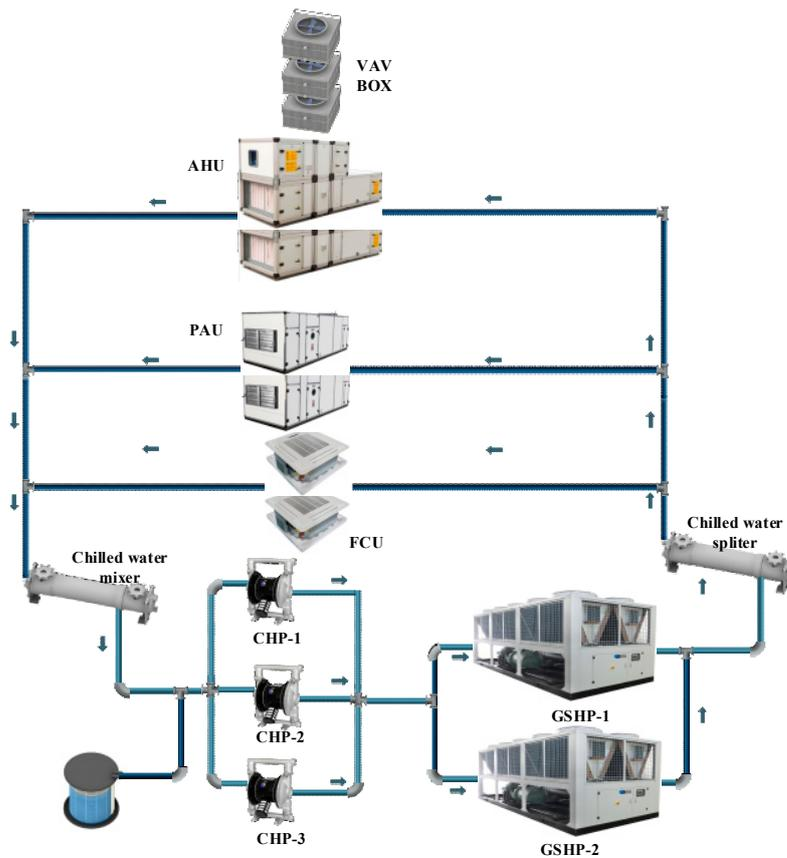
**Figure 6.** HVAC system schematic diagram.
