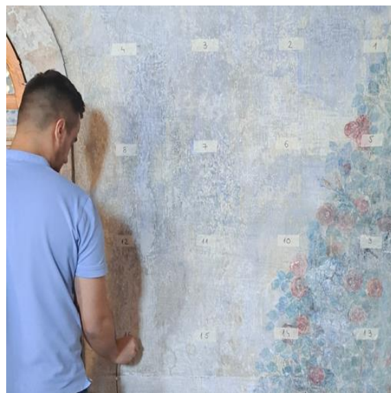
Figure 17. Receiving waves using an accelerometer (inside) (author's photo, 2022).
