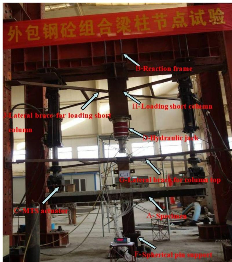
Figure 6. Test setup: (a) the schematic of the test setup; (b) test loading site.
