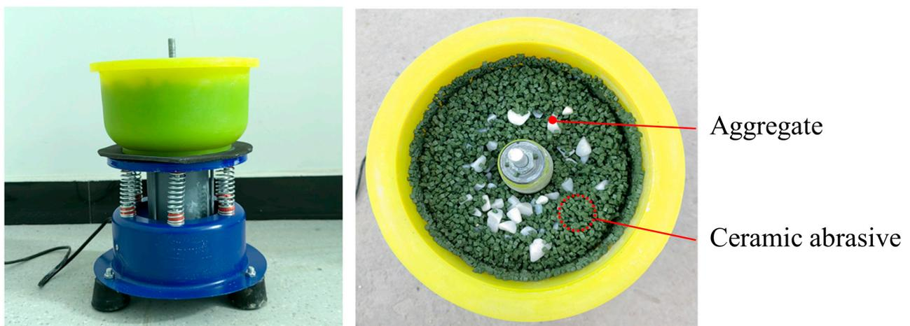
**Figure 1.** Vibration polishing machine to produce aggregates with different roughness.
