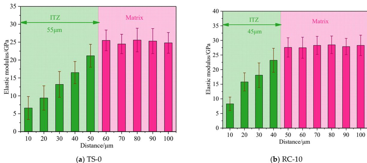
**Figure 9.** Elastic modulus of ITZs.
