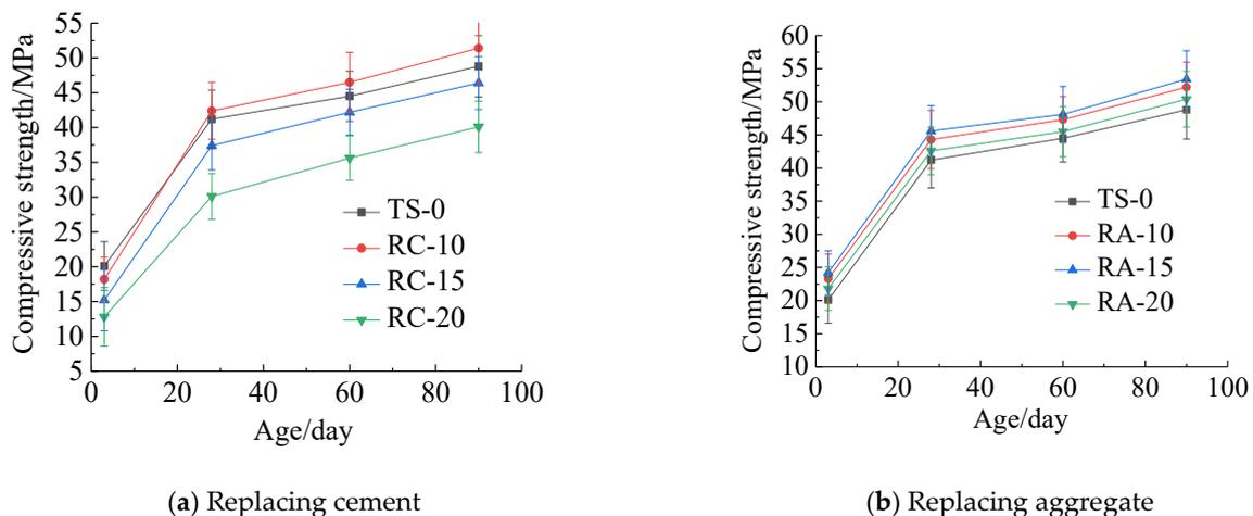
**Figure 4.** Effect of textile sludge on compressive strengths of polypropylene fiber concrete.
