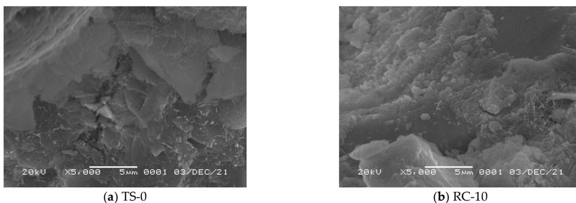
**Figure 6.** SEM images of polypropylene fiber concrete with textile sludge.
