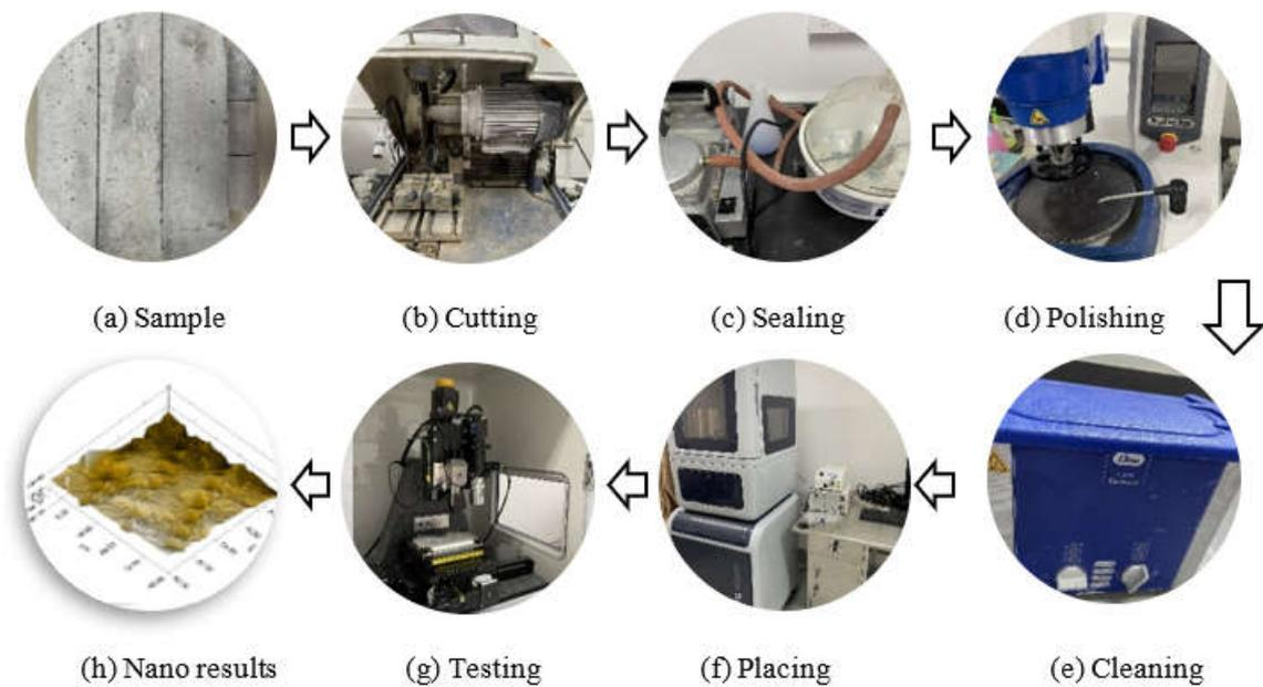
**Figure 3.** Main process of sample preparation and test of nanomechanical properties.
