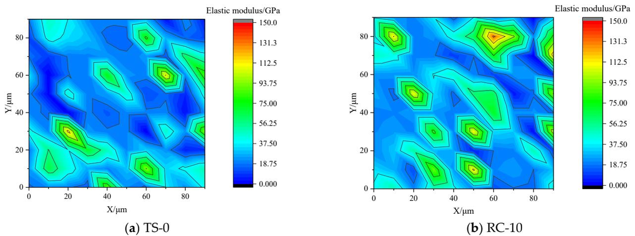
Figure 7. Distributions of elastic modulus of cement matrix.
