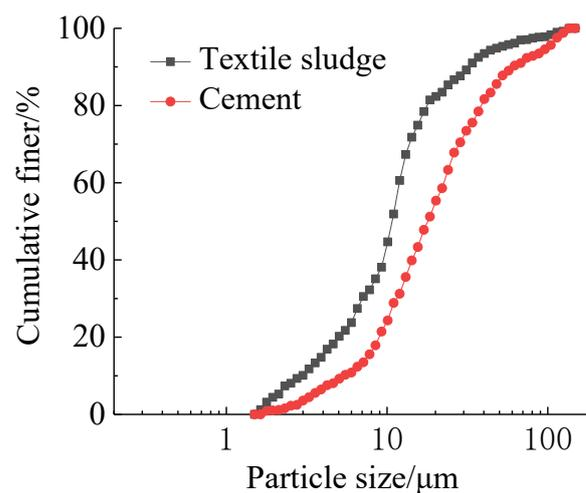
Figure 2. Grading curves of cement and textile sludge.
