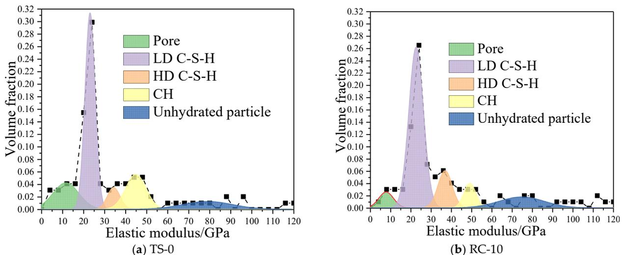
Figure 8. Frequency distributions of elastic modulus of cement matrix.
