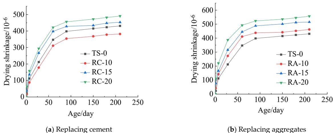
**Figure 5.** Effect of textile sludge on drying shrinkage of polypropylene fiber concrete.
