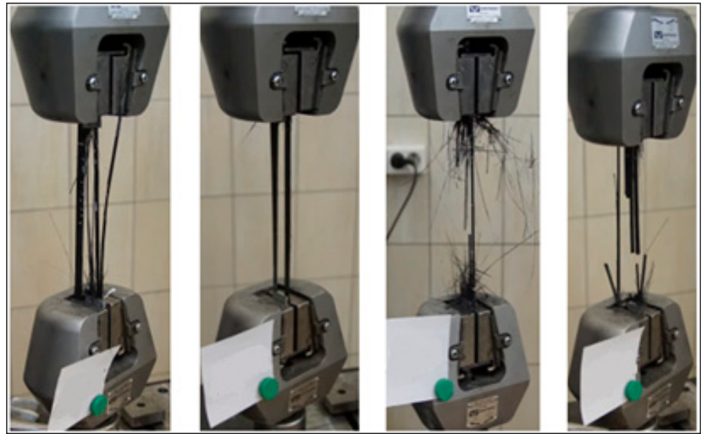
Figure 9. The failure of lamella specimens.
