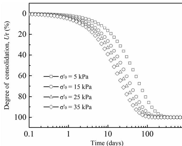
**Figure 10.** Average degree of the proposed model with a variation in  $\sigma'_0$ .
