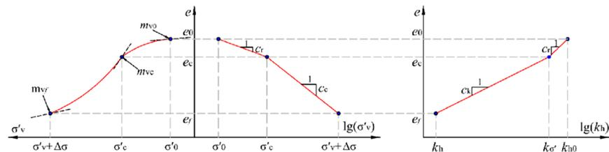
Figure 3. The relationship of  $e$ - $\lg k$  and  $e$ - $\lg \sigma'_v$ .
