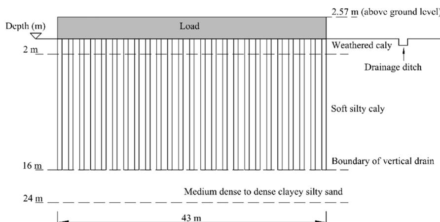
Figure 11. Project details of the Muar clay embankment in Malaysia [17].
