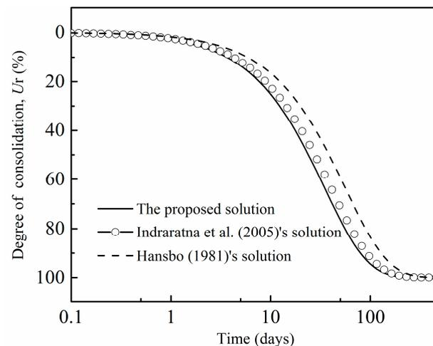
**Figure 5.** Comparison between the proposed model and solutions (from the literature [3,17]).
