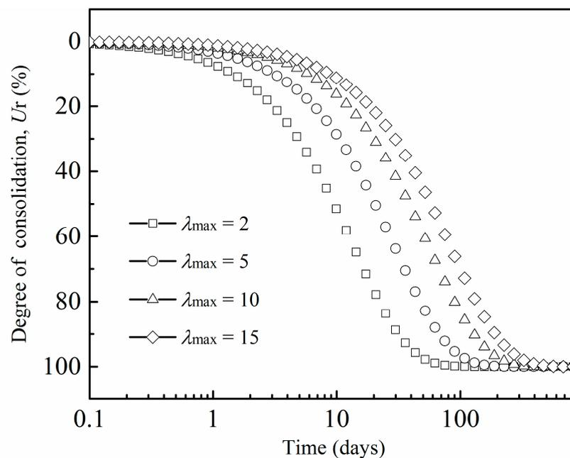
**Figure 6.** Average degree of the proposed model with variation in  $\lambda_{\max}$ .
