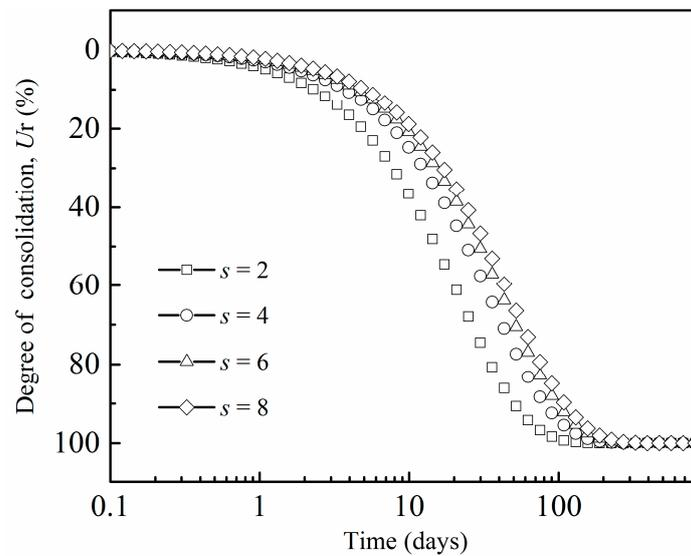
**Figure 7.** Average degree of the proposed model with a variation in  $s$ .
