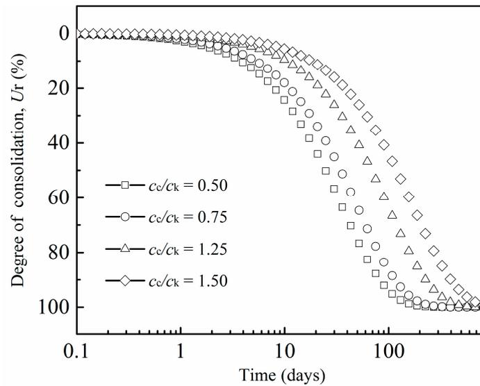
**Figure 9.** Average degree of the proposed model with a variation in  $c_c/c_k$ .
