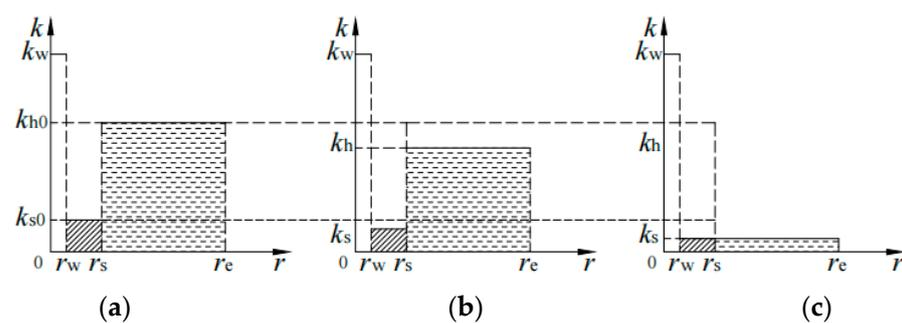
Figure 2. Radial distribution of the permeability coefficient. (a)  $t = t_0$ . (b)  $t = t$ . (c)  $t = t_\infty$ .
