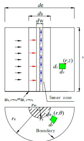
**Figure 1.** Consolidation model for vertical drains including smears.
