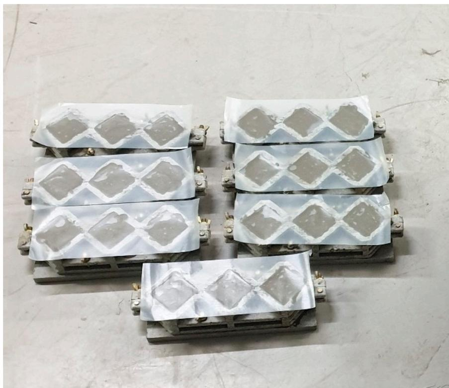
**Figure 2.** Production of specimens.
